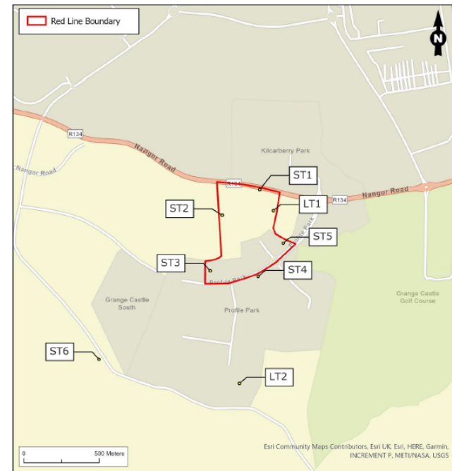
Figure 9.2: Noise Measurement Locations (LT positions were unattended monitoring positions and ST positions were attended monitoring positions)
