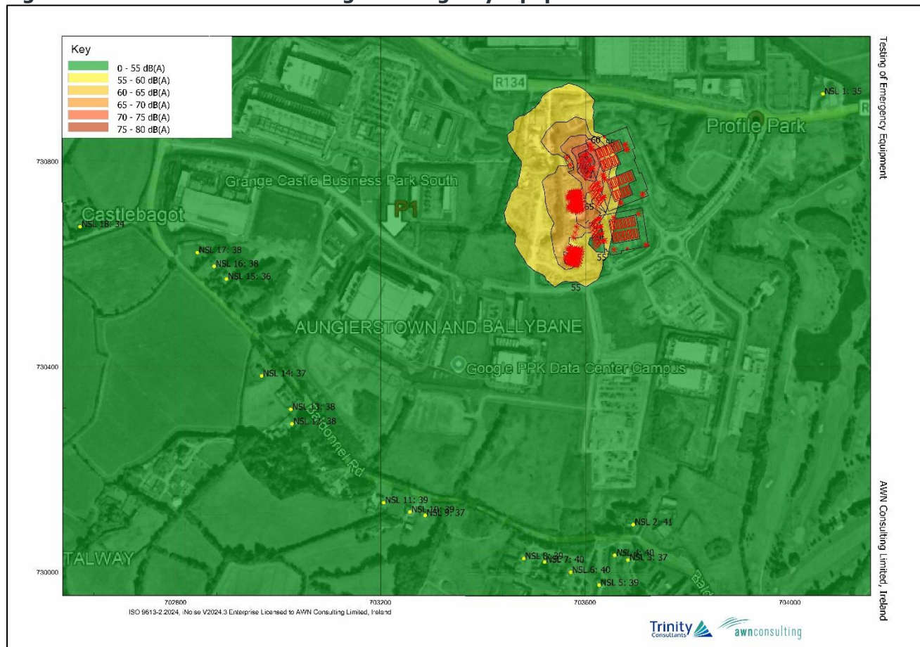
Figure 4-2 Noise contour of Testing of Emergency Equipment
