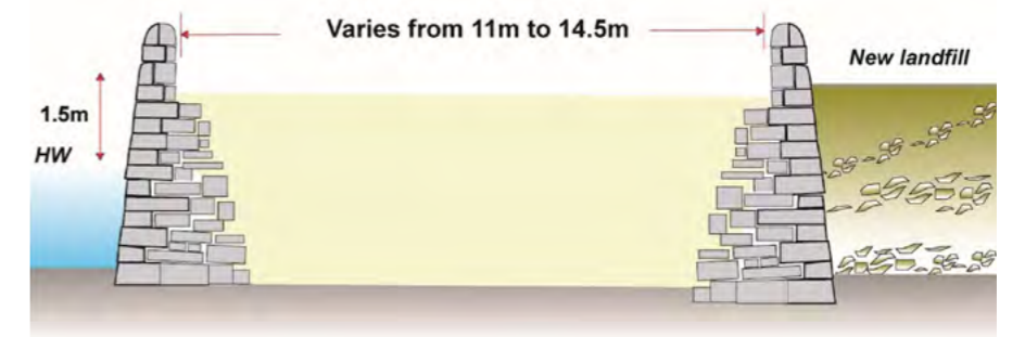
Cross section between Pigeon House precinct and Ringsend (Drawn at exposed section near disused sewerage outfall) Source: Southgate for DPC
