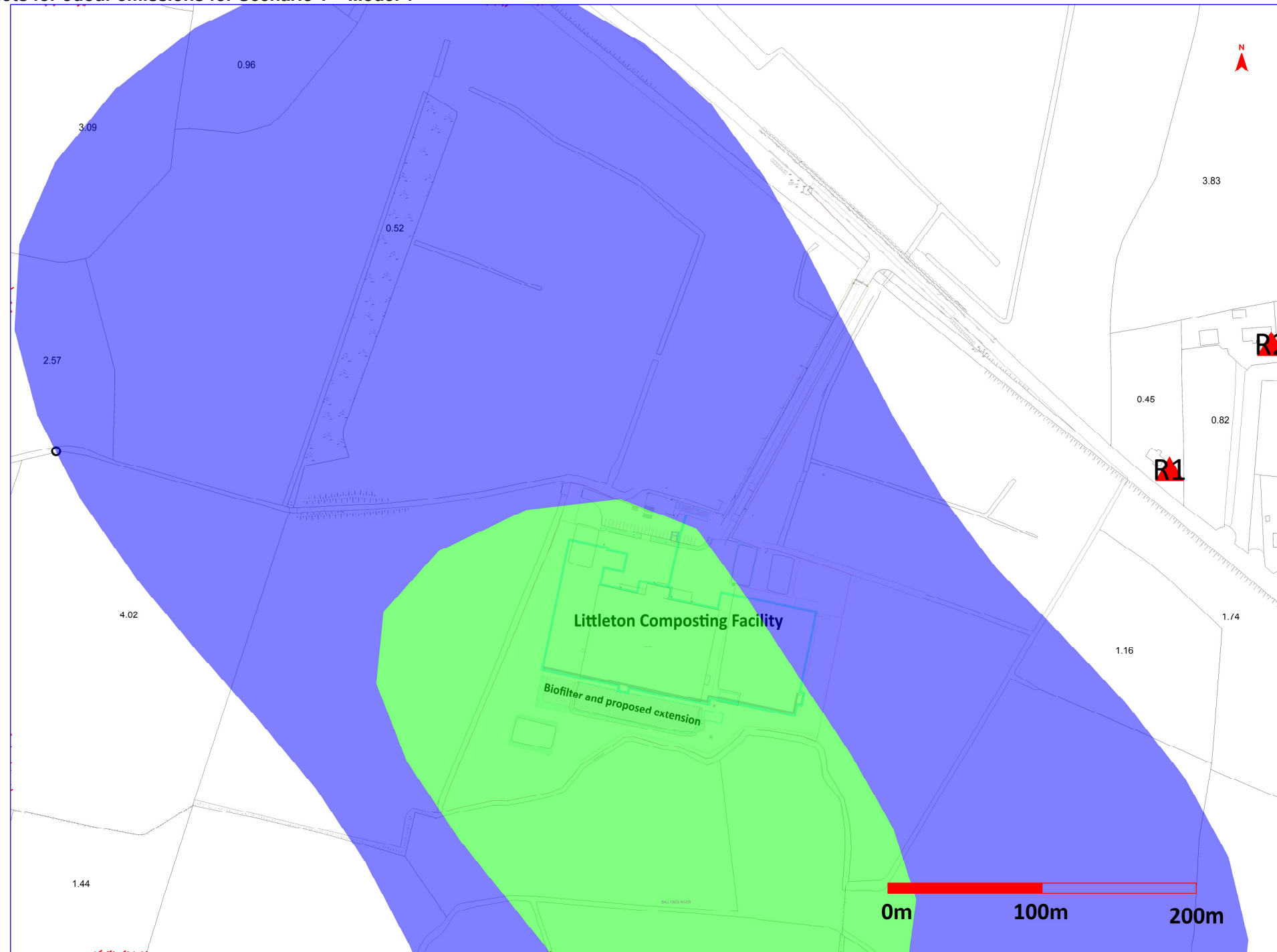
Figure 7.2. Predicted odour emission contribution of proposed Acorn Recycling Composting facility odour sources for Model 1 to odour plume dispersal for an odour concentration of less than or equal to 3.0 O uE /m 3 ( — ) & 6.0 O uE /m 3 ( — ) for the 98 th percentile of hourly averages for worst case meteorological year Oak Park 2017.
