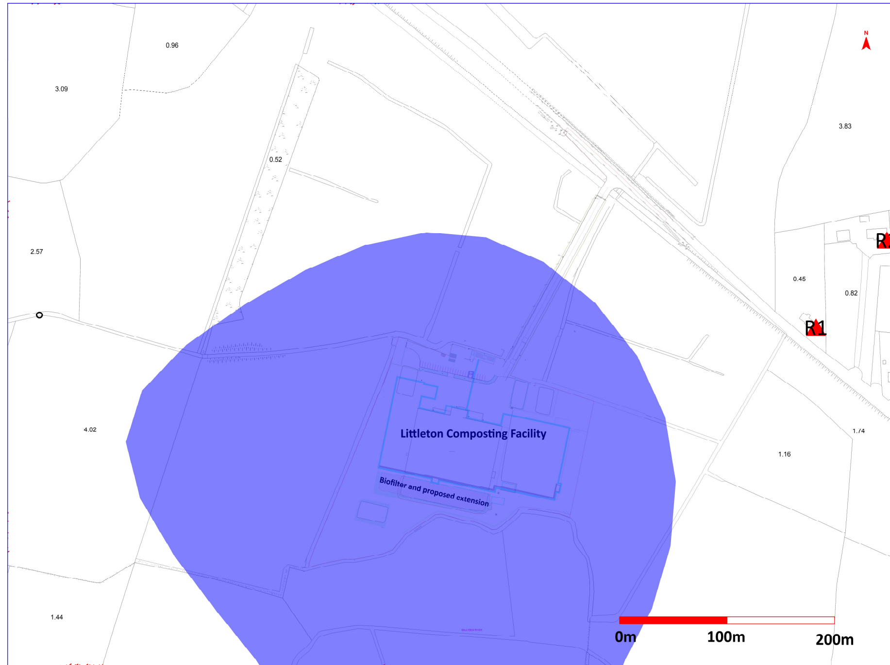
Figure 7.3. Predicted Ammonia emission contribution of proposed Acorn Recycling Composting facility Ammonia sources for Model 2 to Ammonia plume dispersal for an Ammonia concentration of less than or equal to 300\mu\text{g}/\text{m}^3 (—) for the 100 th percentile of hourly averages for worst case meteorological year Oak Park 2017.
