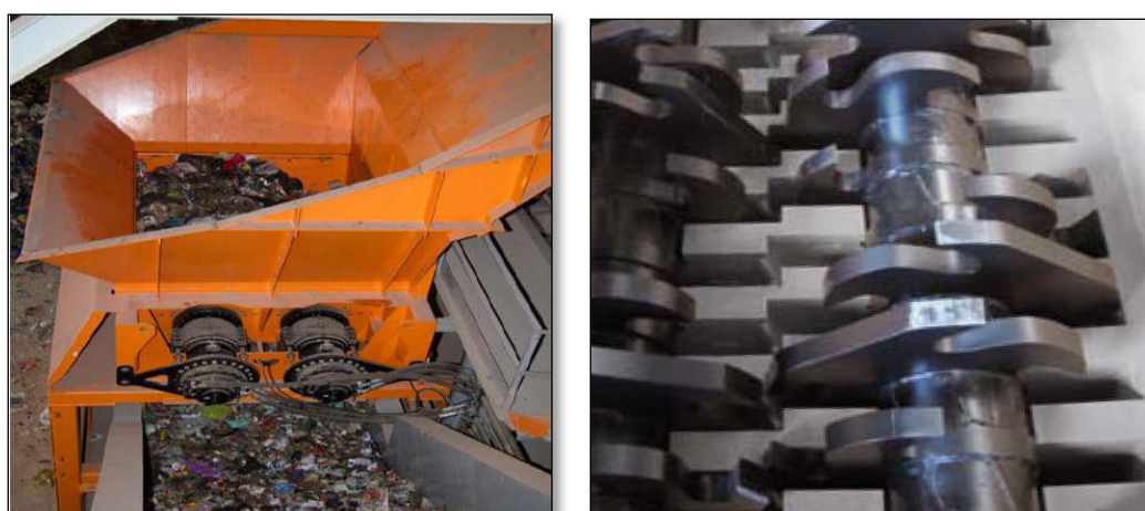
Figure 4-9: Typical example of a bag opener (left) and cutting shaft arrangement (right)
