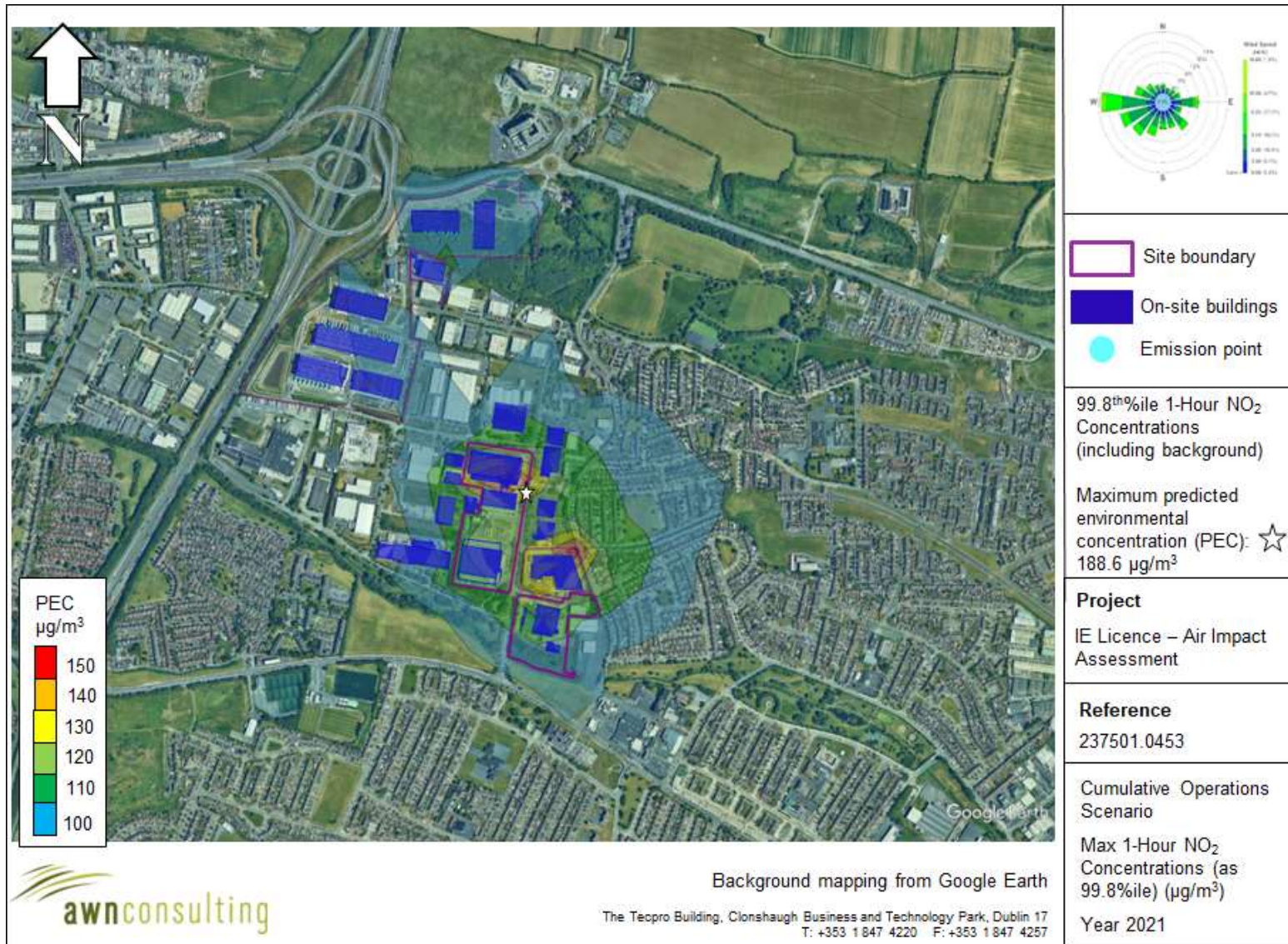
Figure 9 Cumulative Assessment - Maximum 1-Hour NO 2 Concentrations (as a 99.8 th ile) (µg/m 3 ) (including background concentrations)
