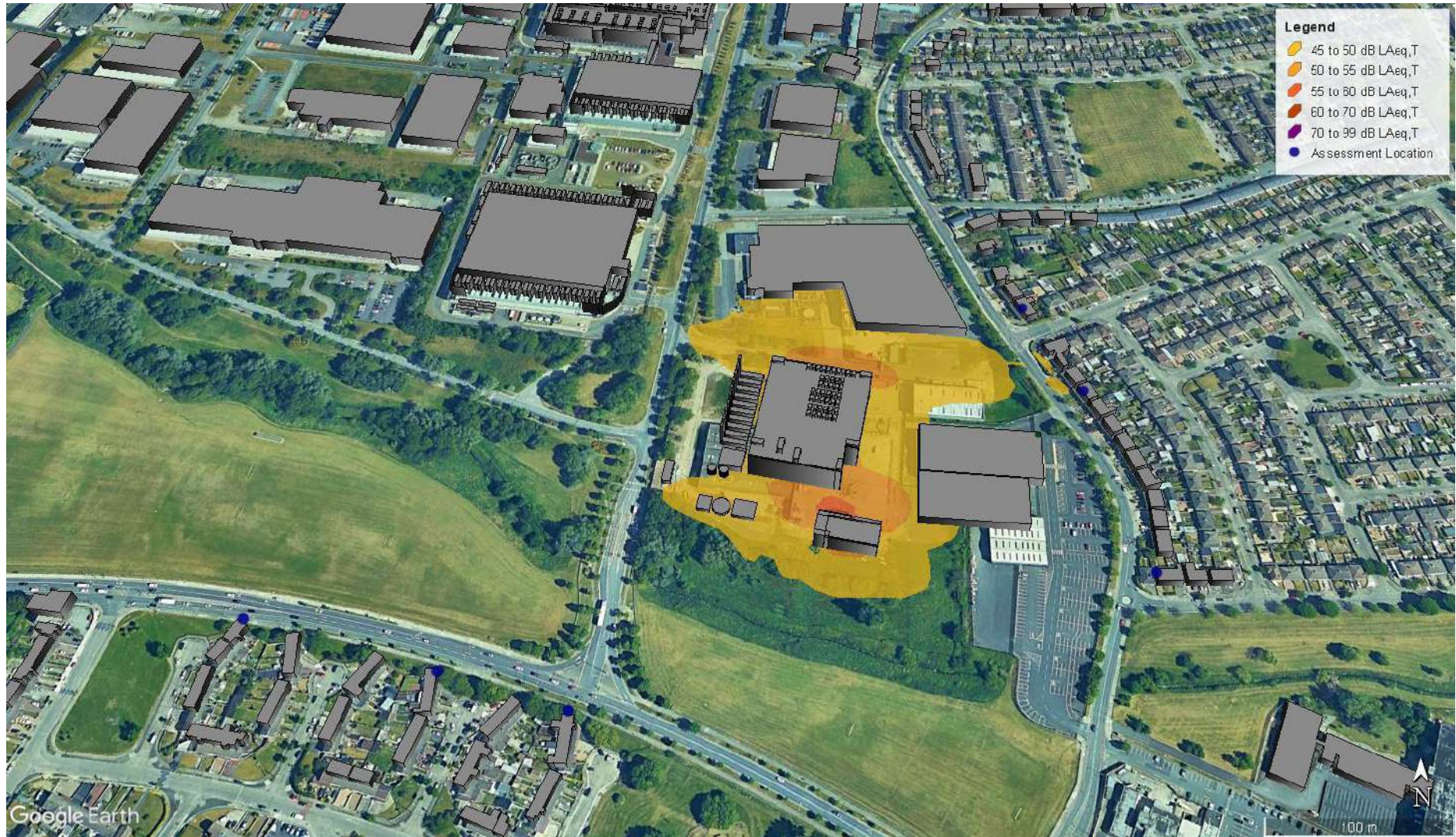
Figure 5 Scenario A – Day to Day Operations Noise Contour – Extent of 35 dB(A) Contour
