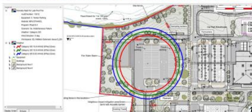
Figure 5-23 Contour plot for a pool fire after instantaneous failure of a tanker at the parking area
