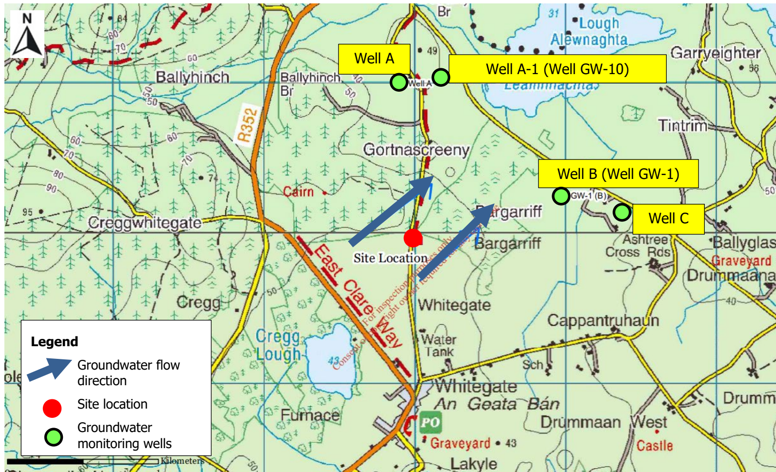
Figure 9: Groundwater flow direction and Groundwater monitoring wells
