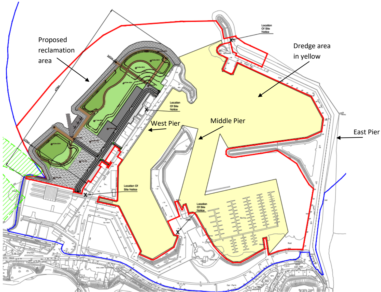
Figure 2. Red line boundary of proposed construction works including site layout (excerpt from planning drawing no. 19934 -5002 Site Layout Plan).
