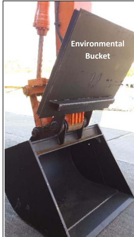
Figure 15 Example of an environmental bucket showing a lid that can be closed to seal contents during lifting.
