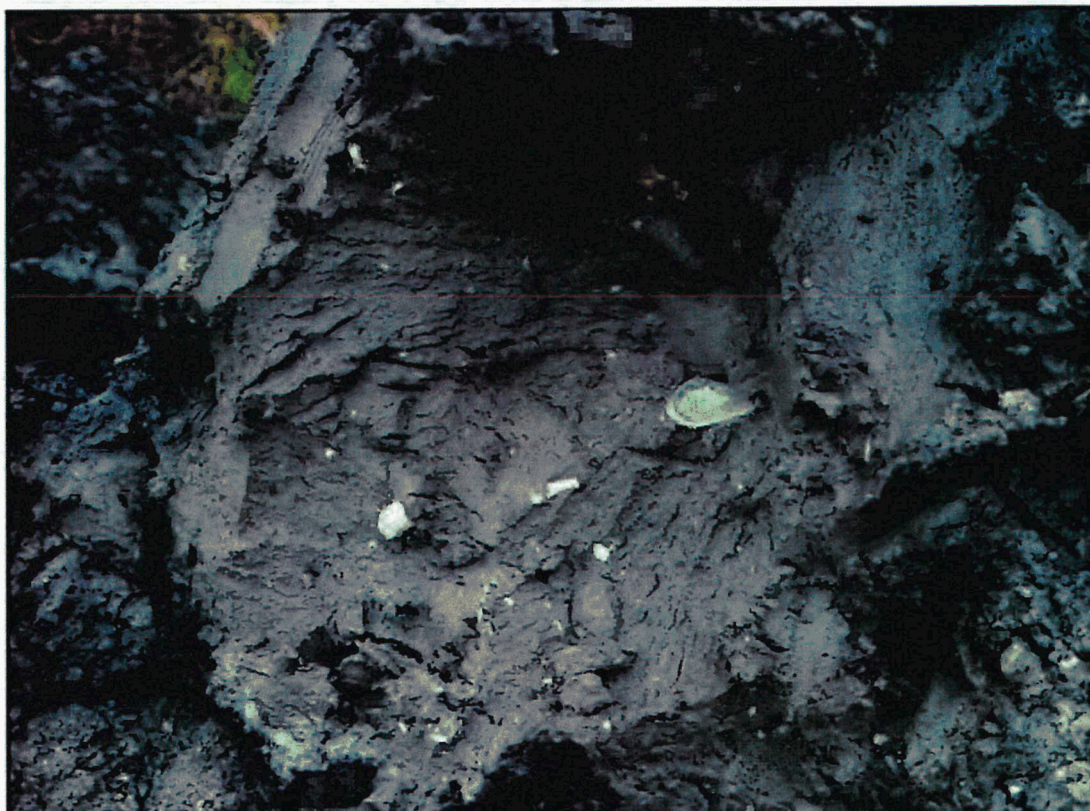
Grey/Black Silt Layer found at base of Trial Pit No.2
