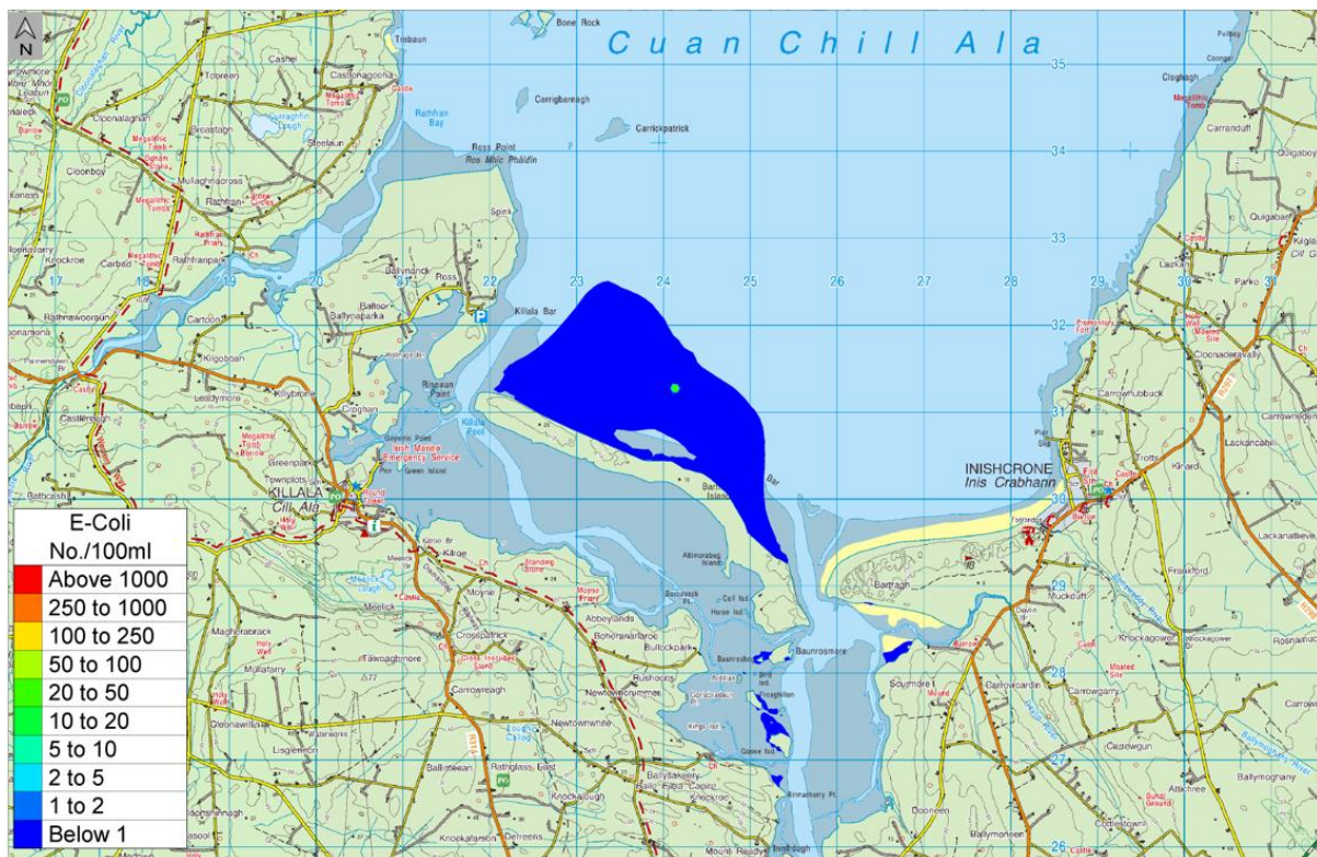
Figure 5-3: Geometric mean E.coli concentrations – Summer die-off rate assessment based on 60-day period
