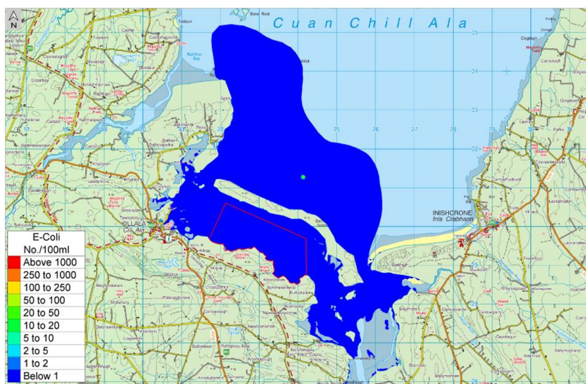
Figure 5-9: Geometric mean E.coli concentrations – Winter die-off rate assessment based on 60-day period
