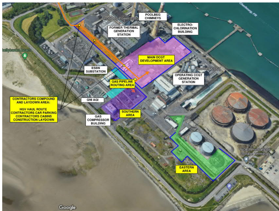
Figure 3.4: Aerial View of ESB Poolbeg Generating Station looking Northwest showing the Designation of the OCGT Development's Work Areas
