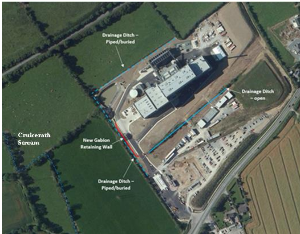
Figure 11.5. Location of drainage ditches within the site boundary and location of Cruicerath Stream.
