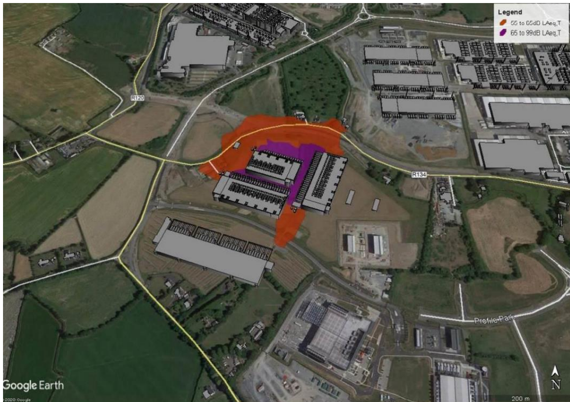
Figure 6.3: Noise Prediction when generators are in operation.
