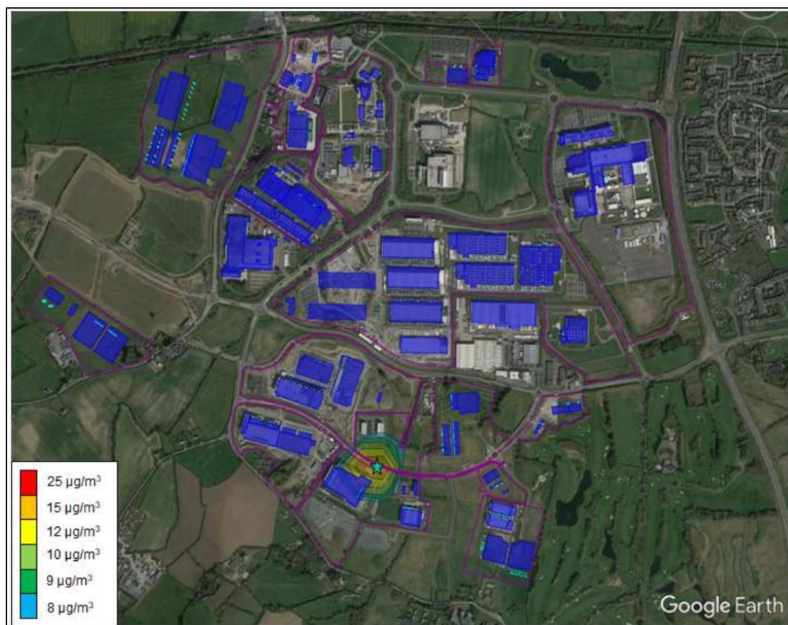
Figure 6.2: Maximum annual mean NO 2 concentration (process contribution) for the worst-case year (2017). The purple lines indicate installation/facility boundaries. [Source: Attachment-7-1-3-2 Emissions Impact Assessment, November 2022]
