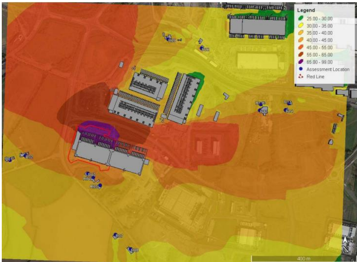
Figure 6.4: Predicted noise levels when back-up generators are in operation (Scenario B) (From Attachment-7-1-3-2-Noise Emissions Impact 8, May 2022).
