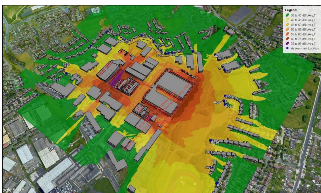
Figure 6.5: Predicted noise levels when generators are in operation (Scenario B).
