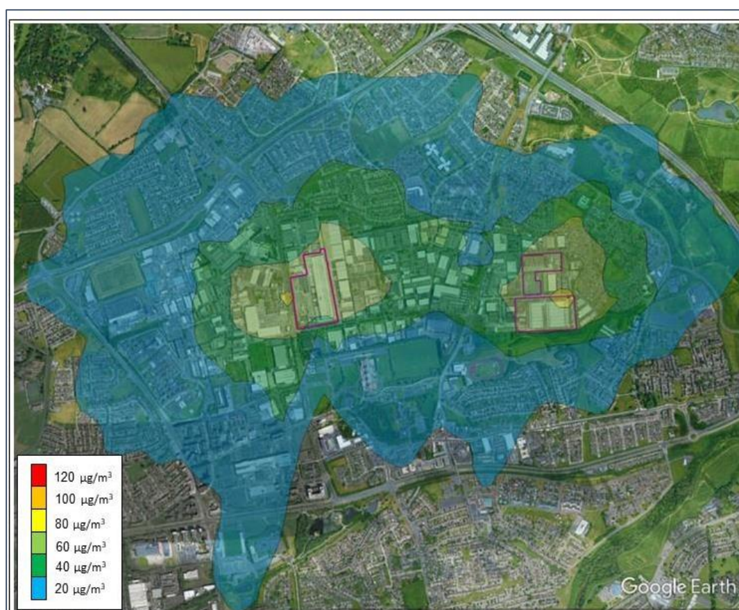
Figure 6.3: Maximum cumulative 1-hour NO 2 concentration (process contributions) for the worst-case year (2018).
