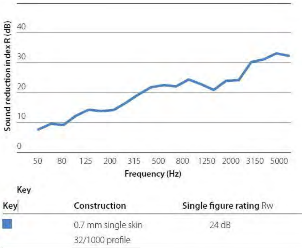
Figure 9-2 – Acoustic Performance of Steel Clad Building Material
