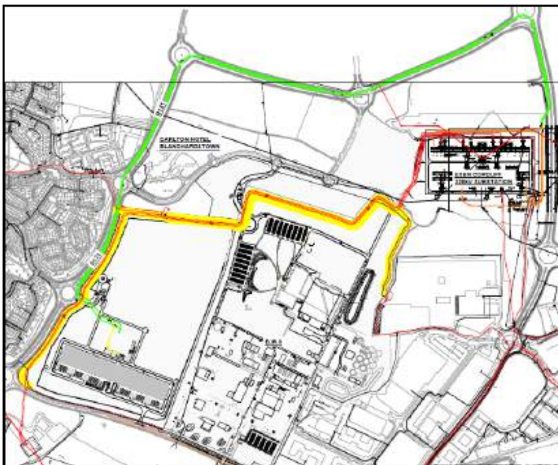
Figure 3.2 220kV Transmission Line Route Option 1 (green line), the location of the permitted Building A and Location of Existing Corduff 220kV Substation (Source: Clifton Scannell Emerson Associates August 2017)
