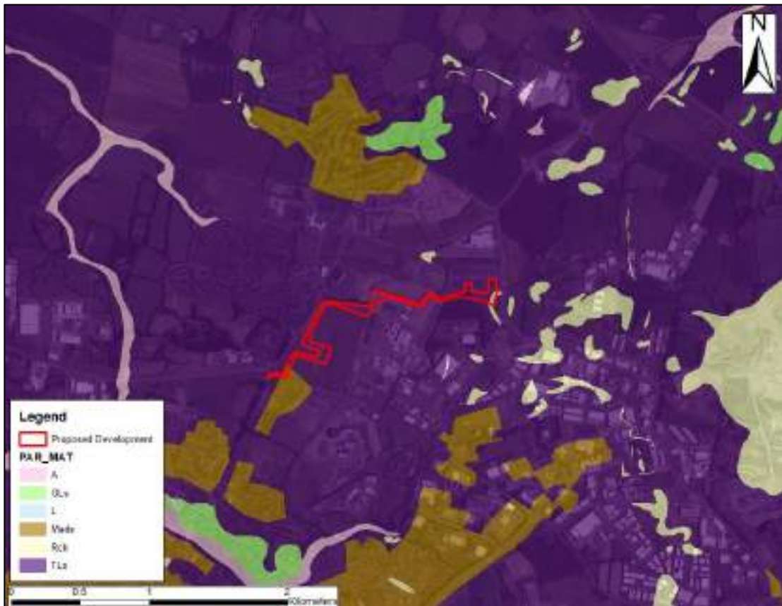
Figure 5.2 Subsoils map for the Proposed Development site (boundary indicated in red) (GSI, 2019)
