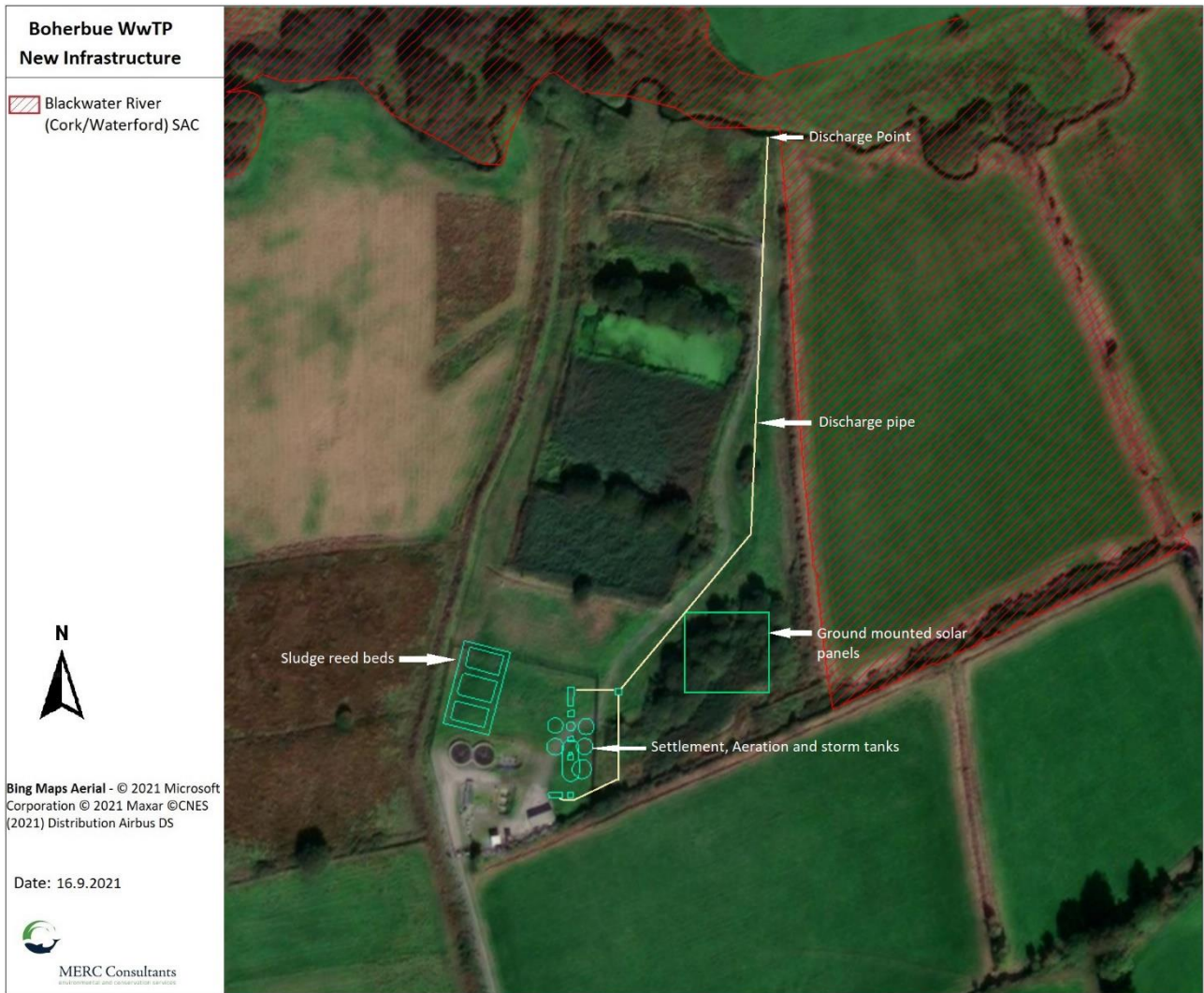
Figure 4.2. Overview of proposed new site infrastructure.
