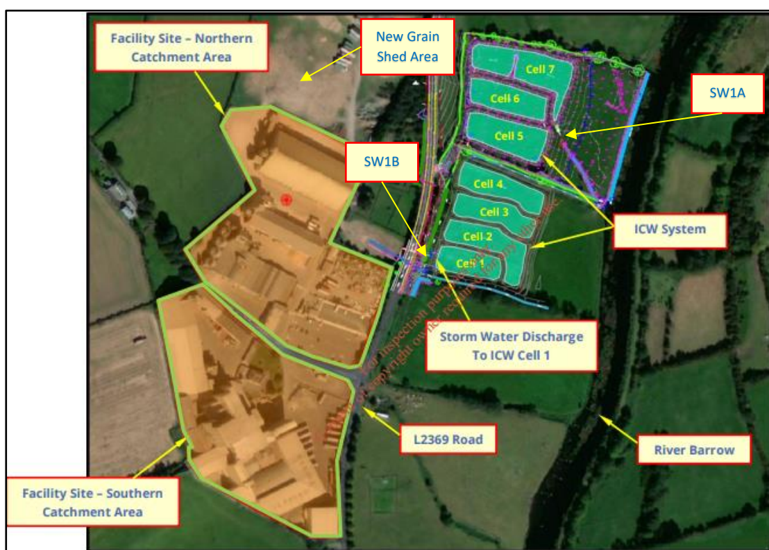
Figure 6.1: William Connolly stormwater catchment area and ICW management system. Source: Figure 1 of Attachment 5 of licence application P1069-01, Titled ' Connolly's Red Mills, Integrated Constructed Wetland (ICW) System ', dated November 2021. Update to Figure by licensing inspector to include SW1A and SW1B for clarity purposes.
