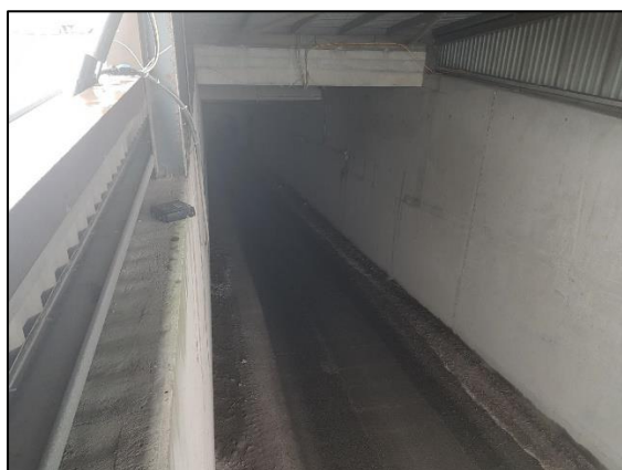
Plate 4.2 Placement of Pettersson at mine entrance, with microphone directed down the mineshaft to detect any bats emerging
