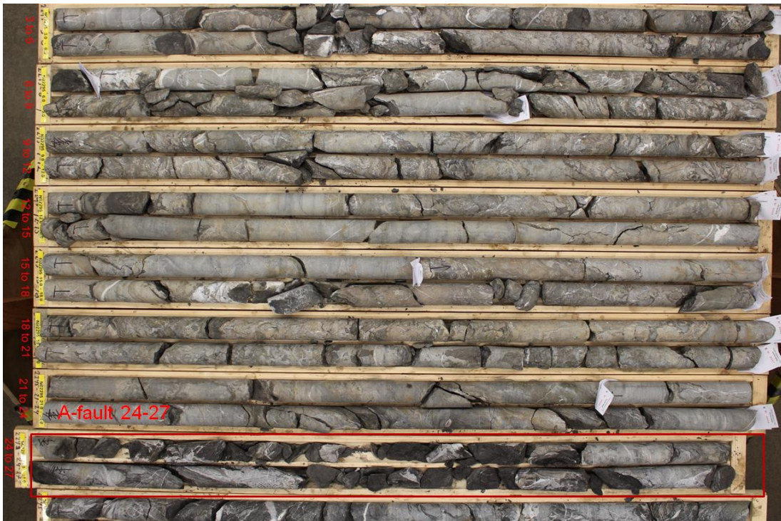
FIGURE 13.15 DRILL HOLE NO2295 SHOWING A-FAULT AT LOCATION APPROX. 24-27 M.
