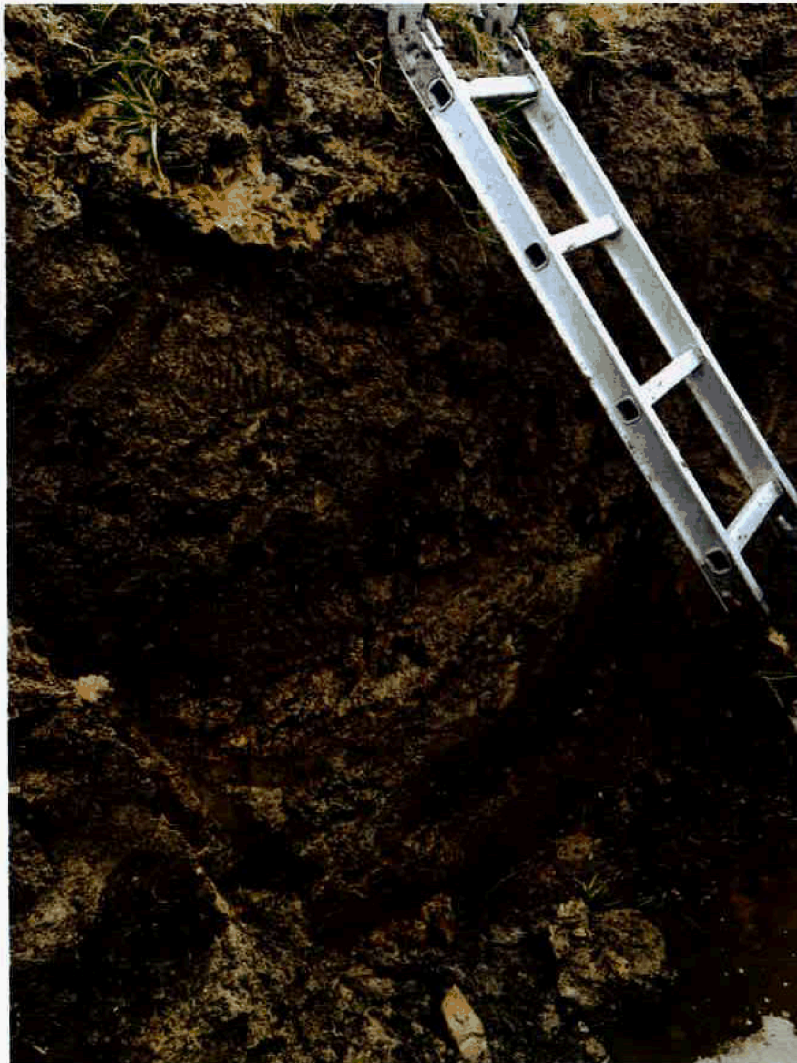
Picture 2 – 2.2m deep Trial Hole
