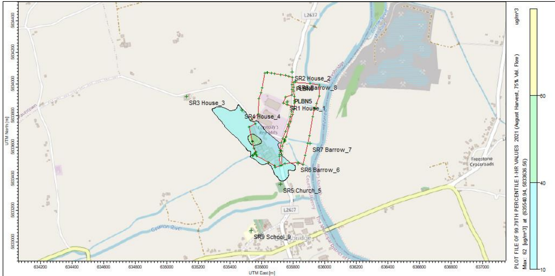
Figure 2-6: Process Contribution SO 2 - Short-Term (1-hr Mean 99.8%ile) for 2021 for August ending harvest at 75% volumetric flow
