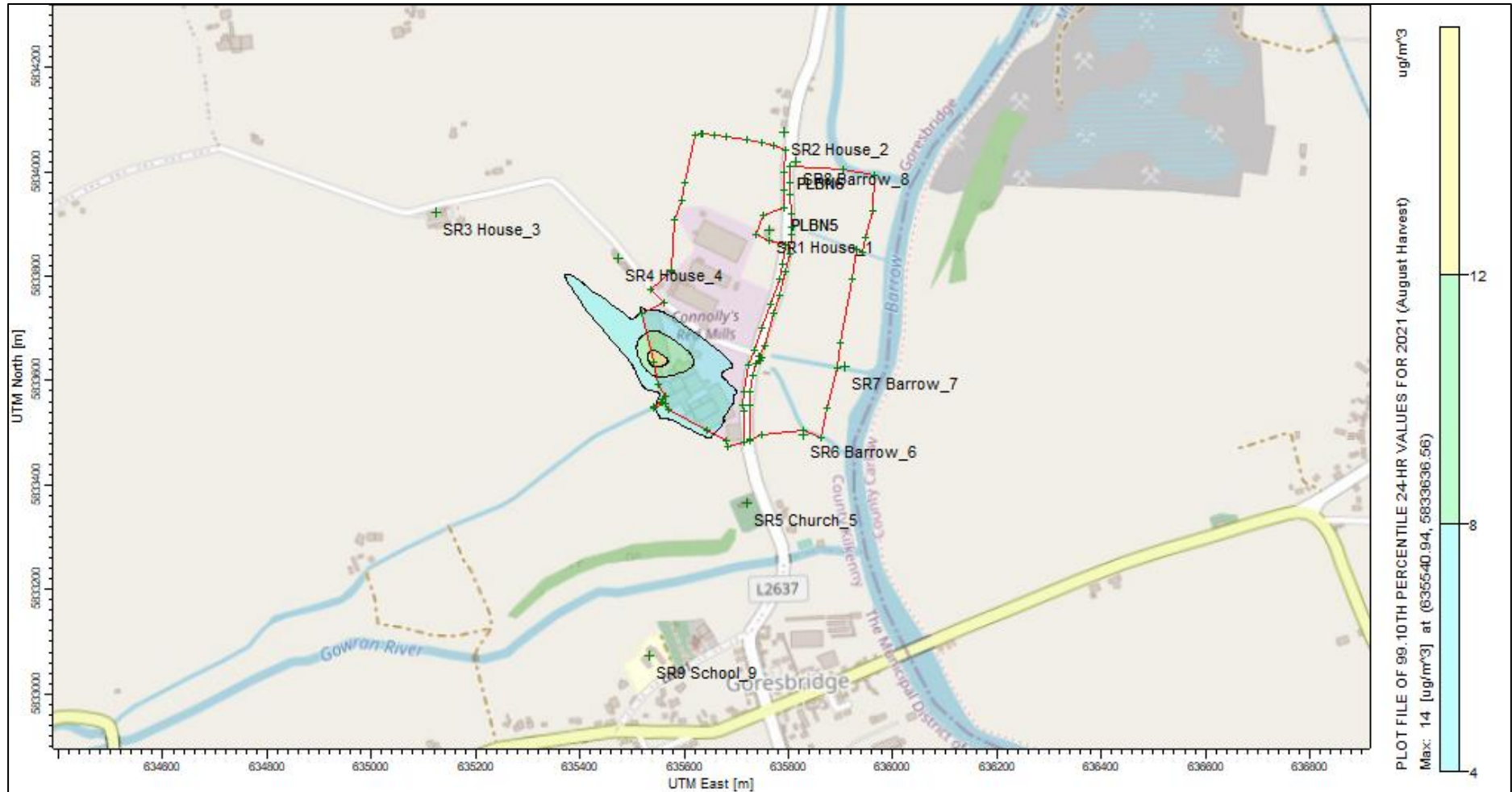
Figure 2-9: Process Contribution SO 2 – Short Term (24-hr Mean 99.10%tile) for 2021 for August ending harvest at 100% volumetric flow
