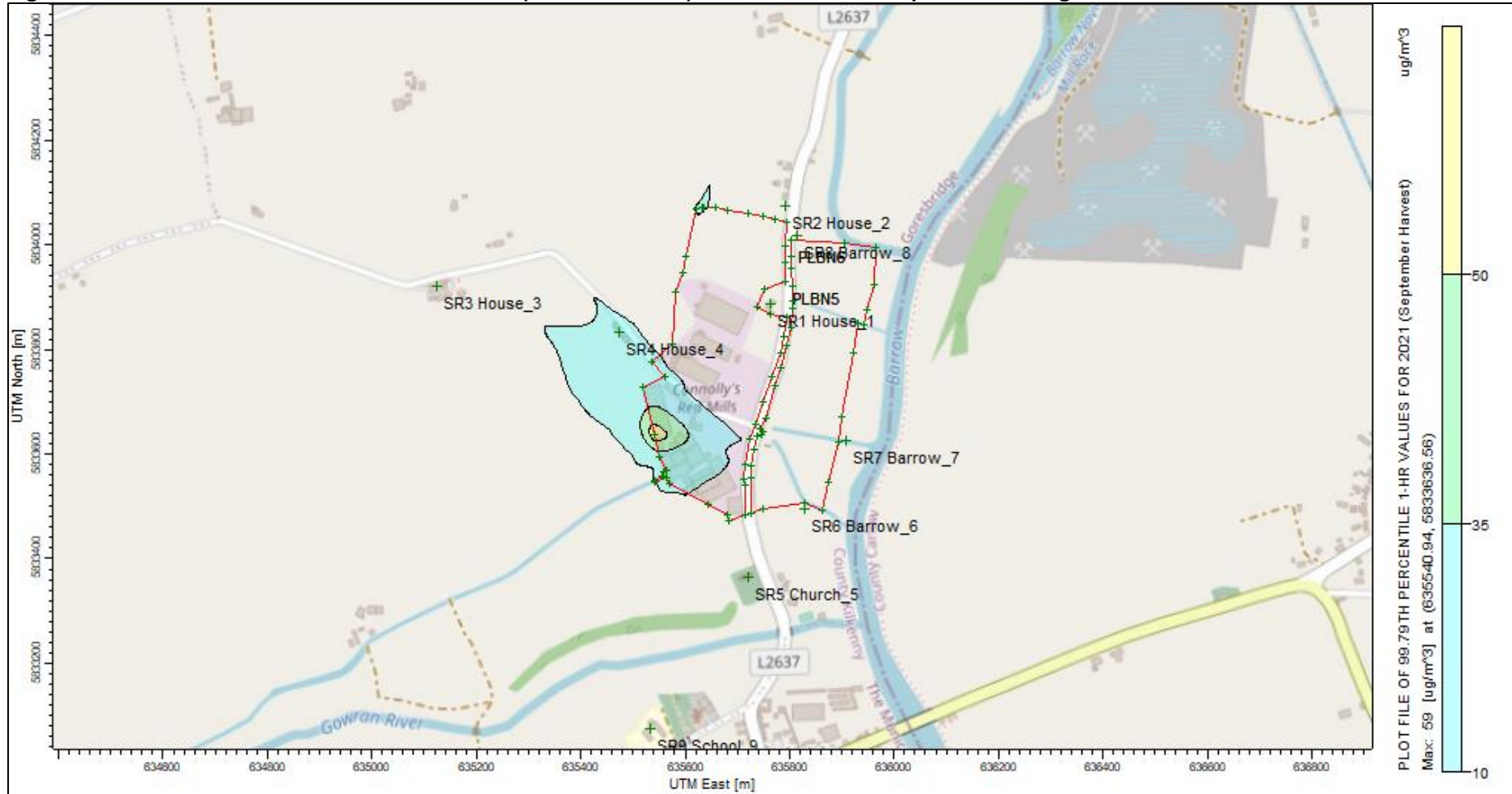
Figure 2-7: Process Contribution SO 2 - Short Term (1-hr-99.79 th ile) Mean for 2021 for September ending harvest at 100% volumetric flow
