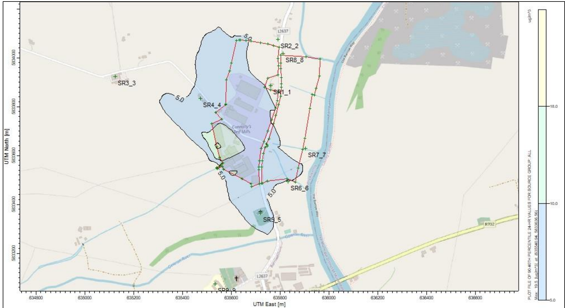
Figure 3-20: Process Contribution PM10 – 24-hr (90.4th%ile) for 2021 for August (2021) ending harvest at 75% volumetric flow
