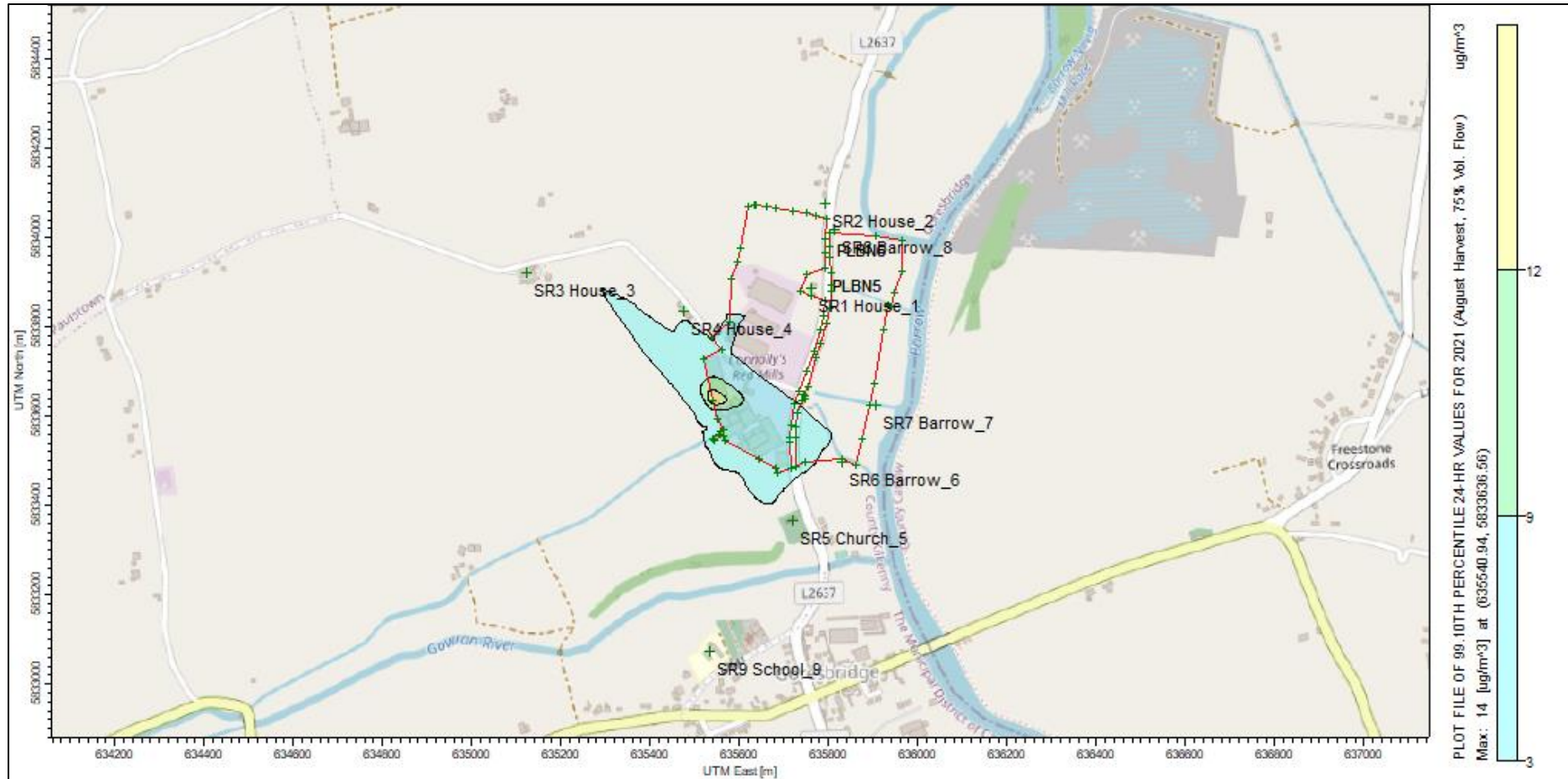
Figure 2-10: Process Contribution SO 2 – Short Term (24-hr Mean 99.10%tile) for 2021 for August ending harvest at 75% volumetric flow
