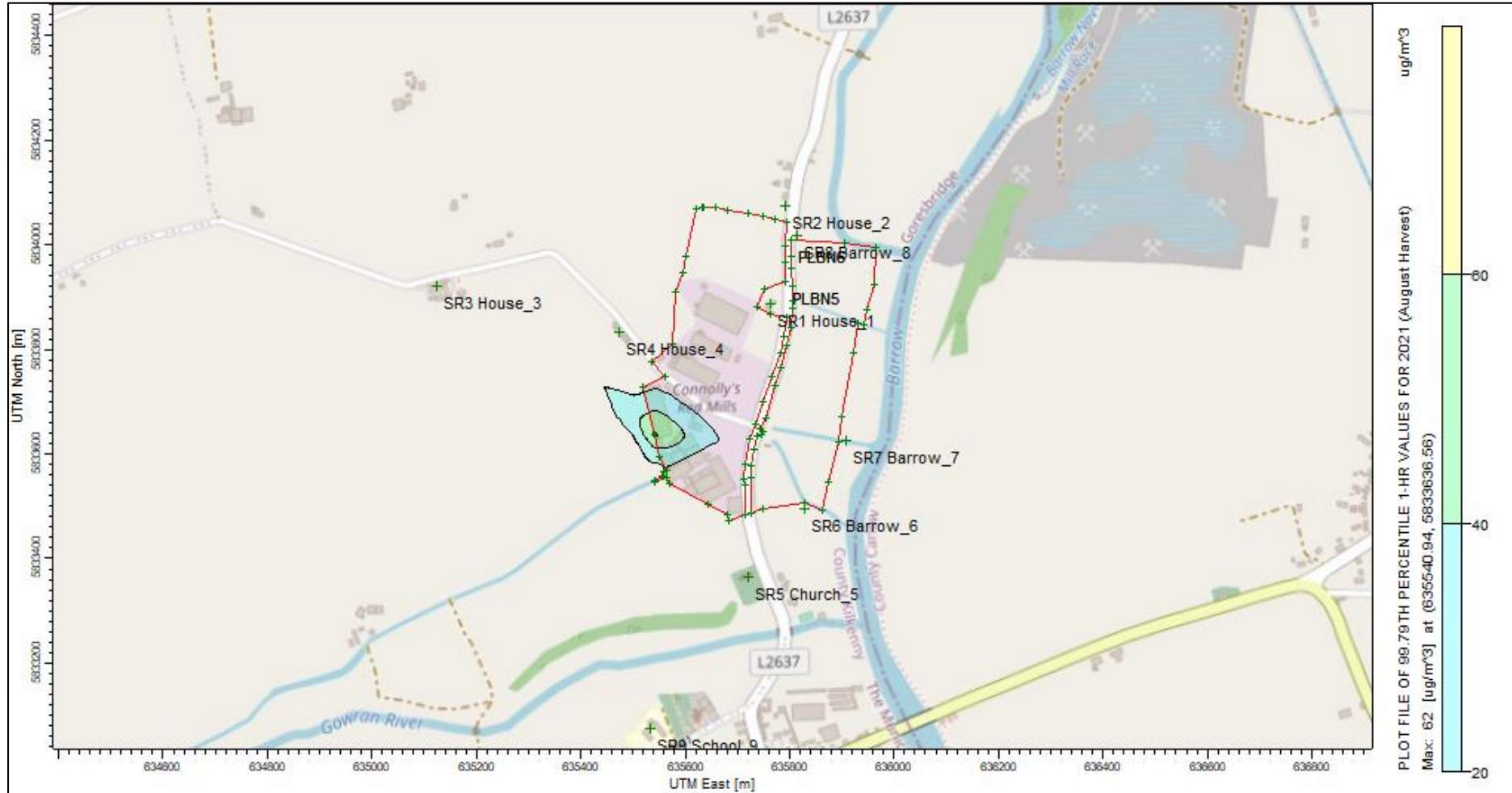
Figure 2-5: Process Contribution SO 2 - Short Term (1-hr-99.79 th ile) Mean for 2021 for August ending harvest at 100% volumetric flow
