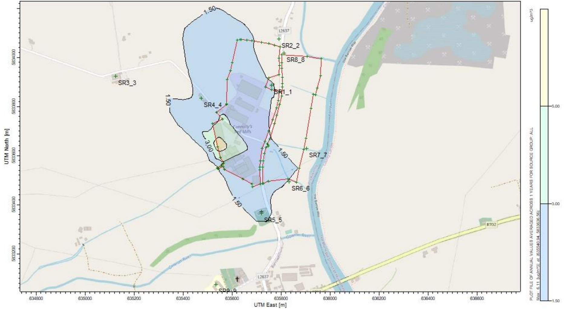
Figure 3-15: Process Contribution PM10 – Annual Mean (90.4th%ile) for 2021 for August (2021) ending harvest at 75% volumetric flow
