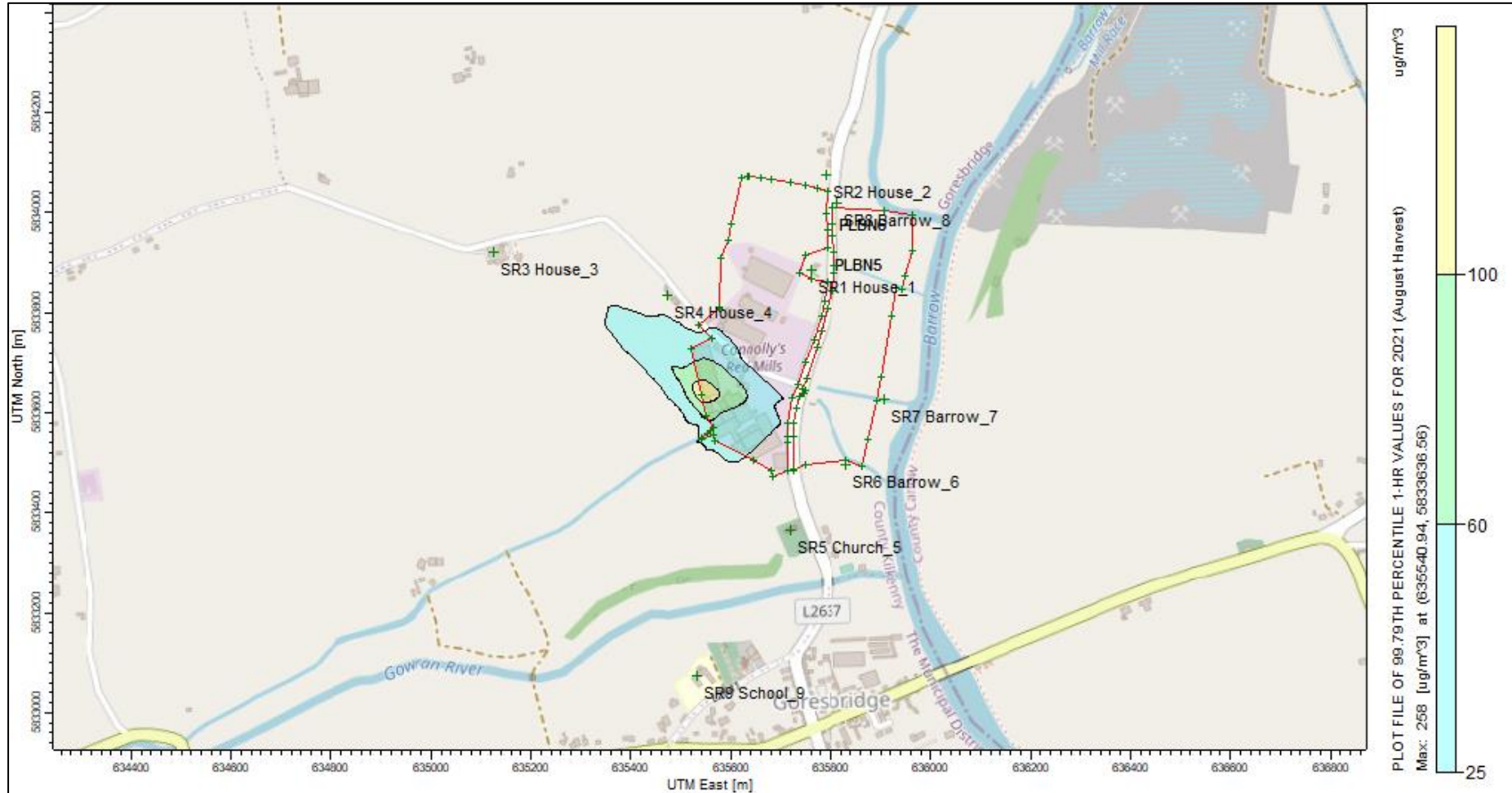
Figure 1-5: Process Contribution NO 2 – Short Term (1-hr-99.79 th ile) for 2021 for August ending harvest at 100% volumetric flow
