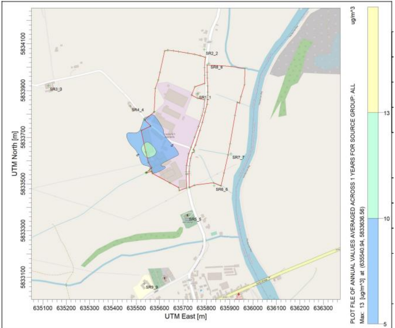
Figure 3-10: Process Contribution PM10 – Annual Mean (90.4th%ile) for 2021 for 12 week harvest at 100% volumetric flow
