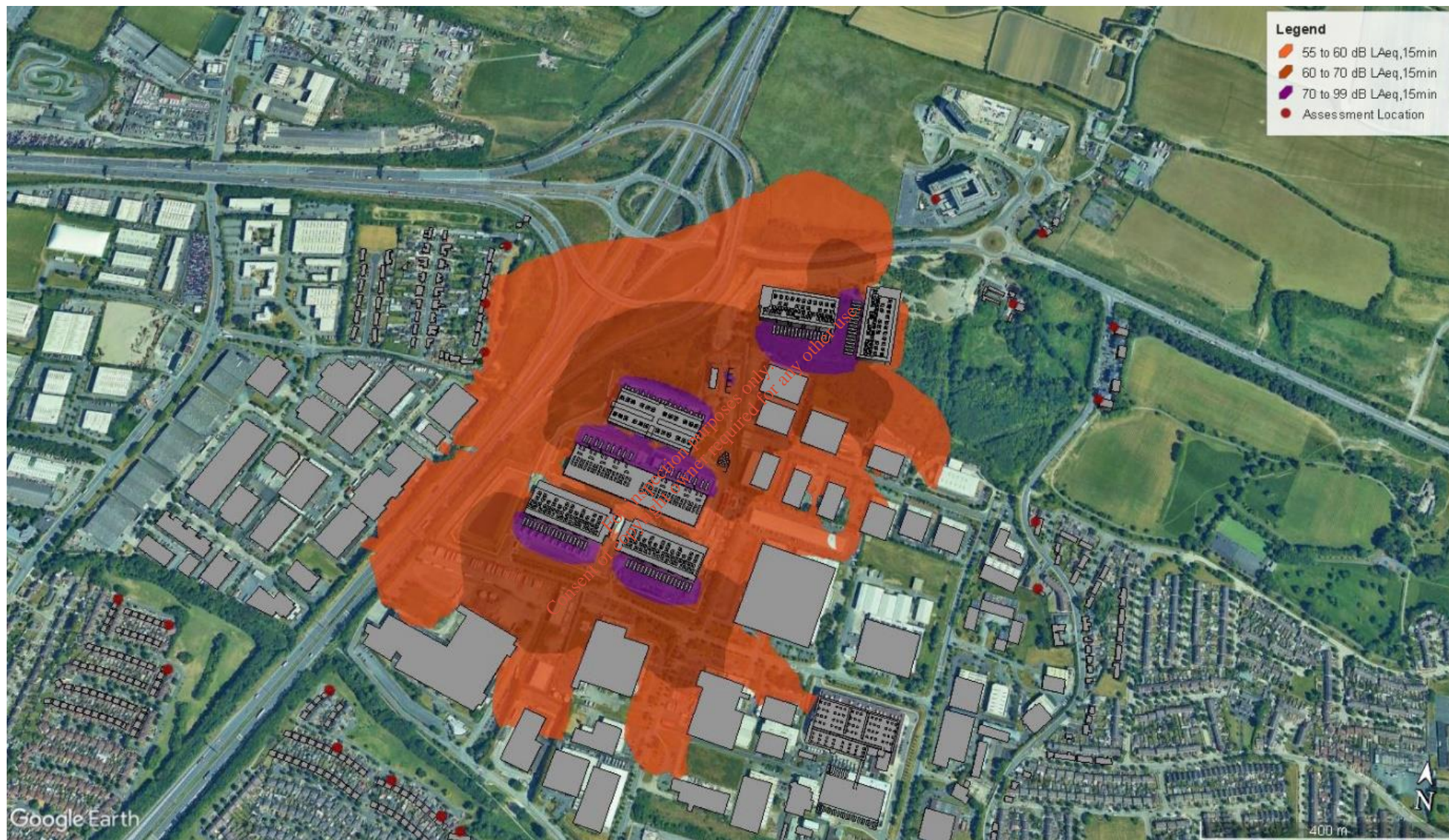
Figure 7 Operational Noise Prediction Contours – Scenario B
