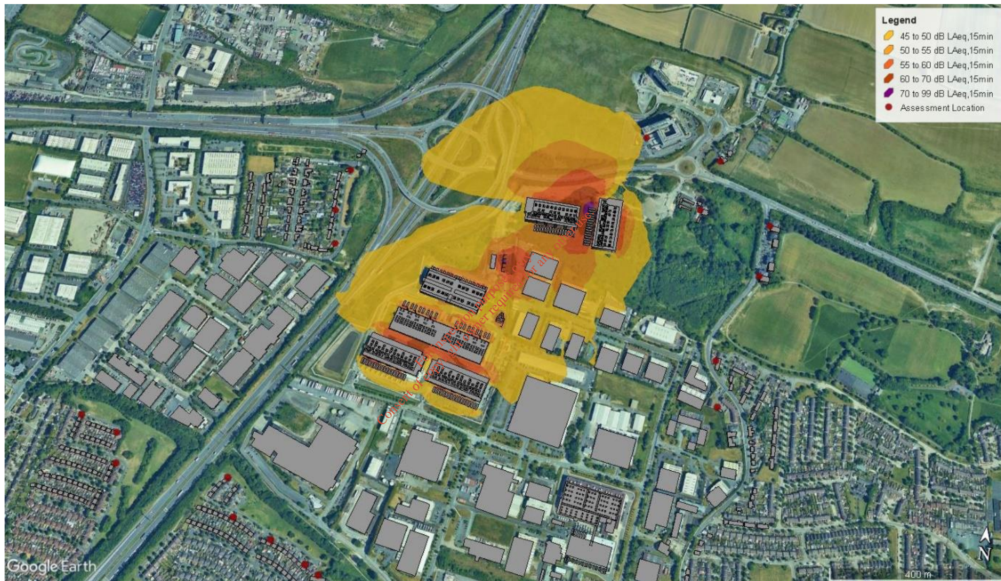
Figure 8 Operational Noise Prediction Contours – Scenario C
