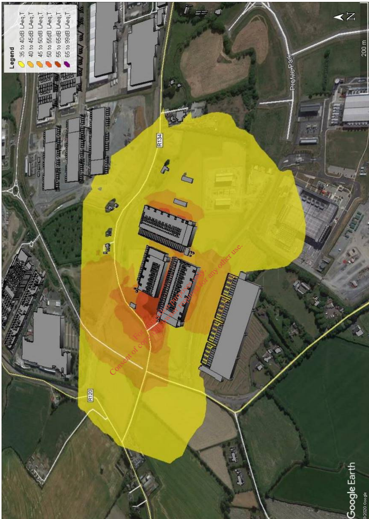
Figure 9.12 Scenario C1 - Proposed Data Centre (current planning application) – Generator Testing Noise Contour (Extent of 35dB(A))
