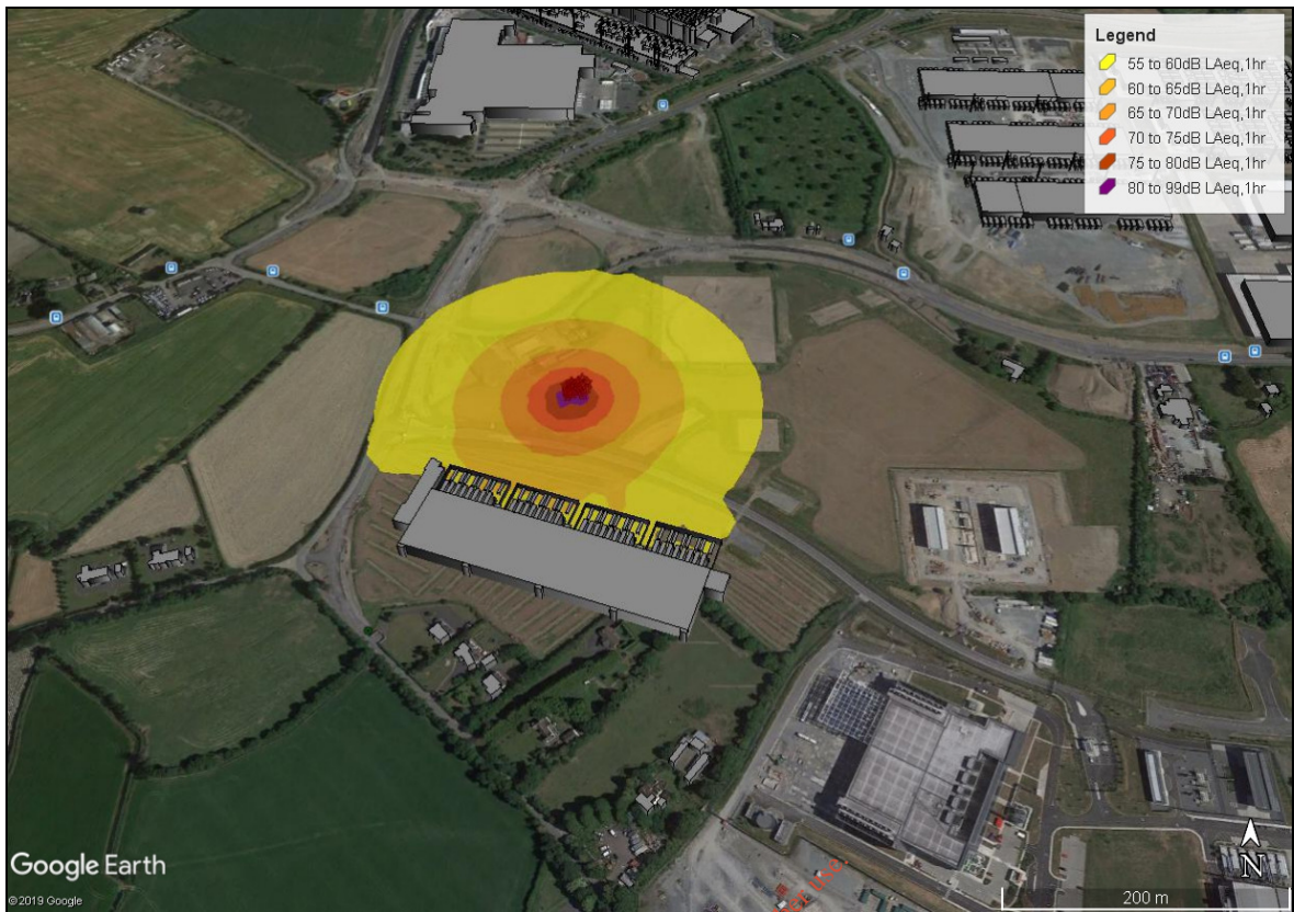
Figure 9.7 Construction noise contour – steel erection.
