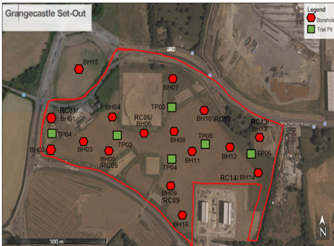
Figure 7.3 Site Investigation Sample Locations (site boundary indicated in red) (Source: OCSC, 2019).
