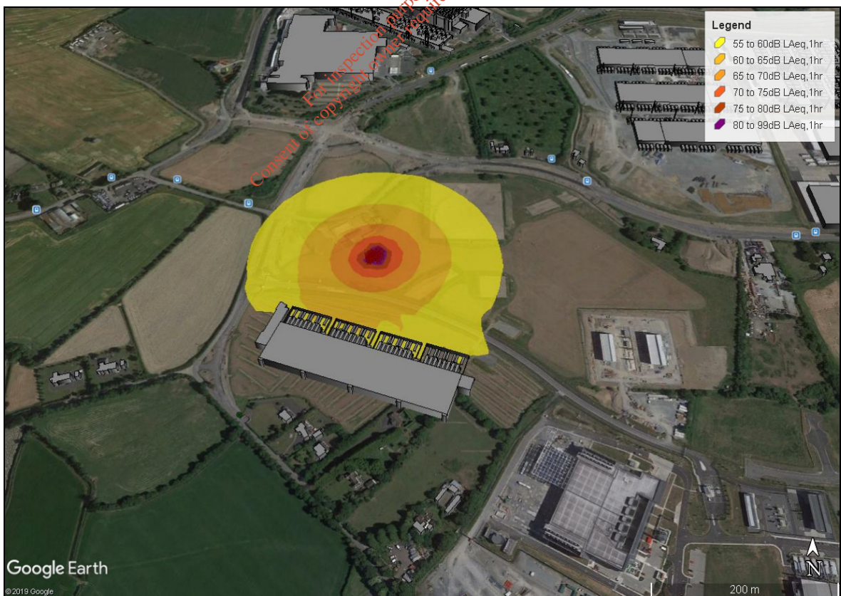
Figure 9.6 Construction noise contour – foundations
