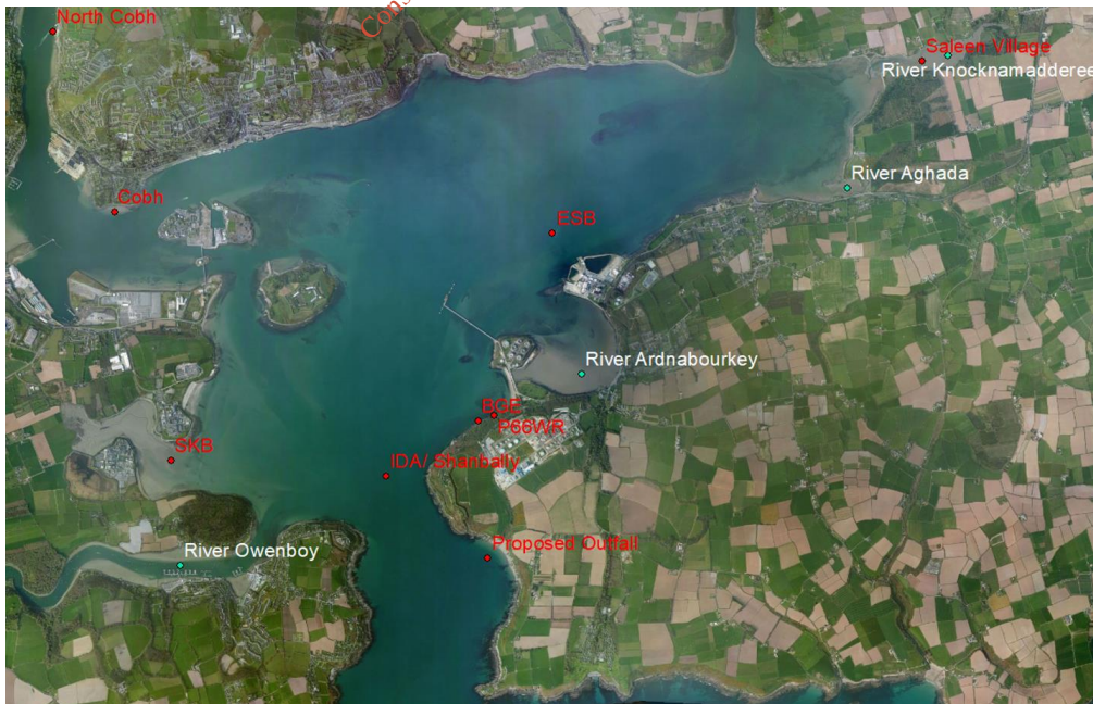
Figure 47: Proposed discharges (fluvial inflows in green, outfalls in red)
