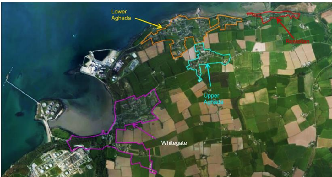
Figure 2: Existing Drainage Areas (Jennings O'Donovan/AECOM Design Report 2015)
