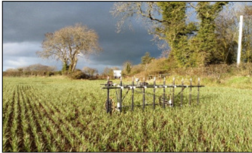
4. Advanced multi-channel gradiometer system for magnetometer survey (manual configuration).
