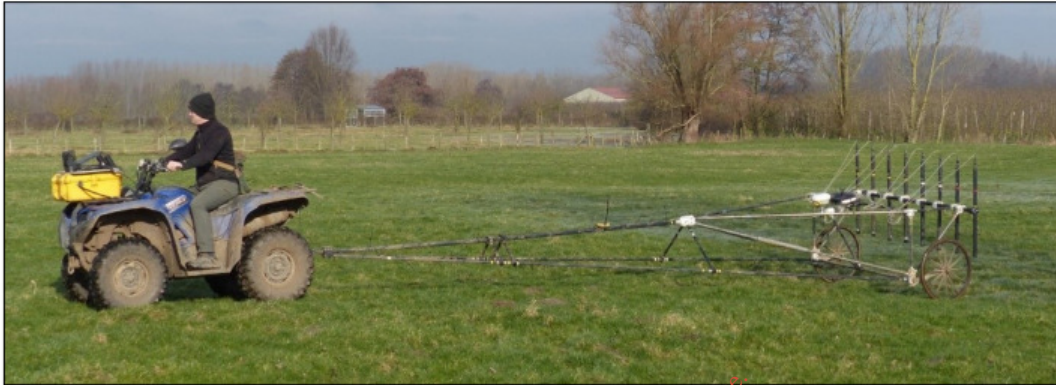
1. Advanced multi-channel magnetometer survey mapping the buried foundation of a 14th century castle (towed configuration with ATV).
