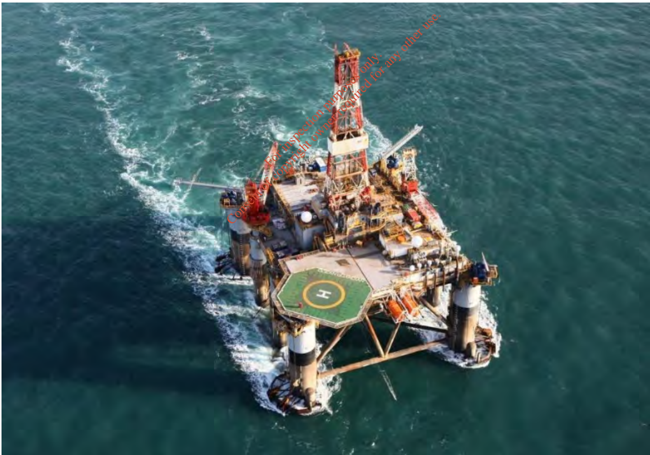
Figure 3.13: Typical semi-submersible drilling rig (MODU)
