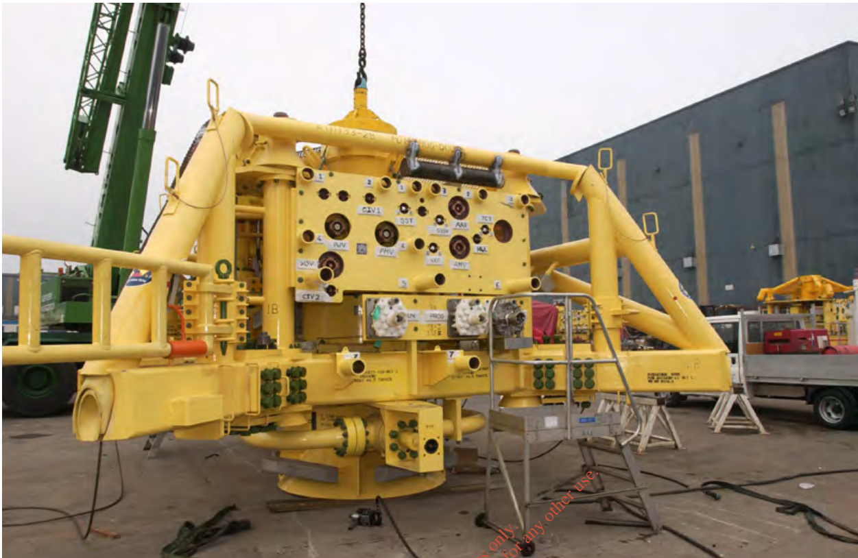
Figure 3.8 Typical subsea Xmas Tree structure
