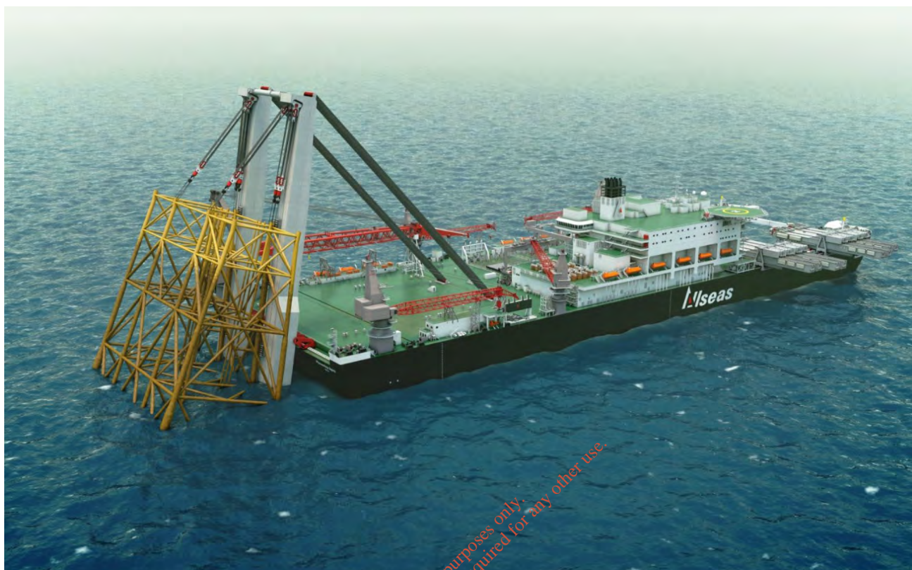
Figure 3.16: Specialist HLV, in this case, Pioneering Spirit , with jacket lifted from the seabed and tilted towards the vessel deck
