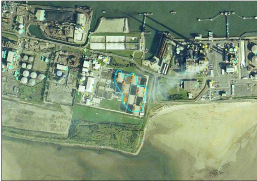
Fig PGGH_Dublin_009.1 Red and orange Envisat PSI points showing an area of subsidence on aerial imagery (Licence No. EN 0047212)
