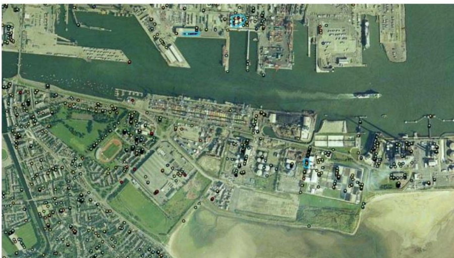
Fig PGGH_Dublin_002.2 shows an image of a 3 km section of the estuary of the River Liffey. ERS PSI point data indicates subsidence in certain parts of the area.
