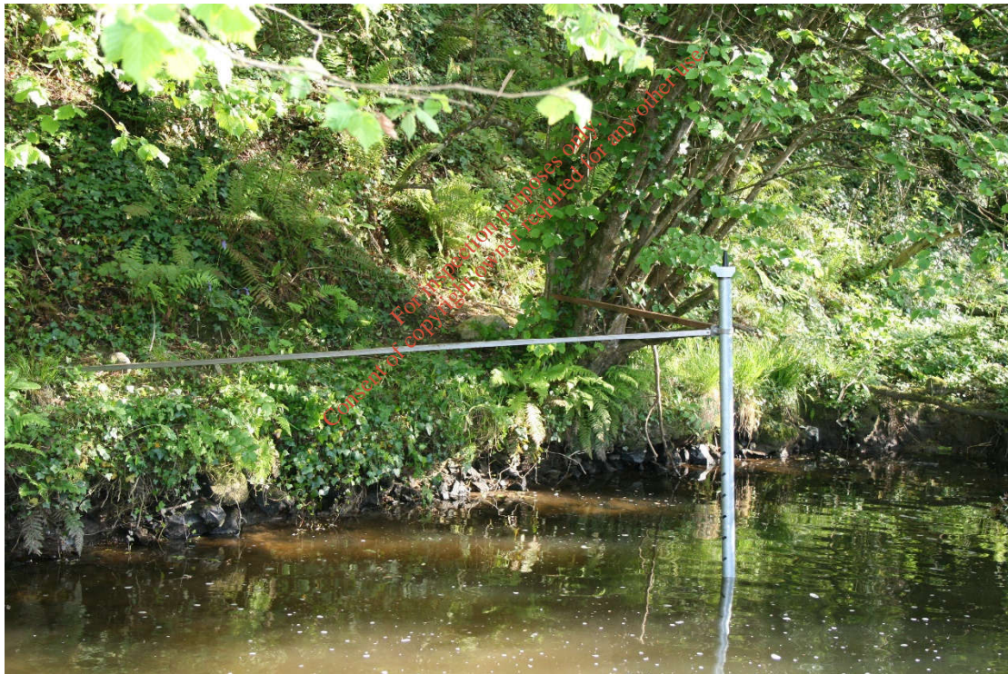
Plate 17. Ecolog 500 monitoring the flow of the river beside site in Kilcurry.
