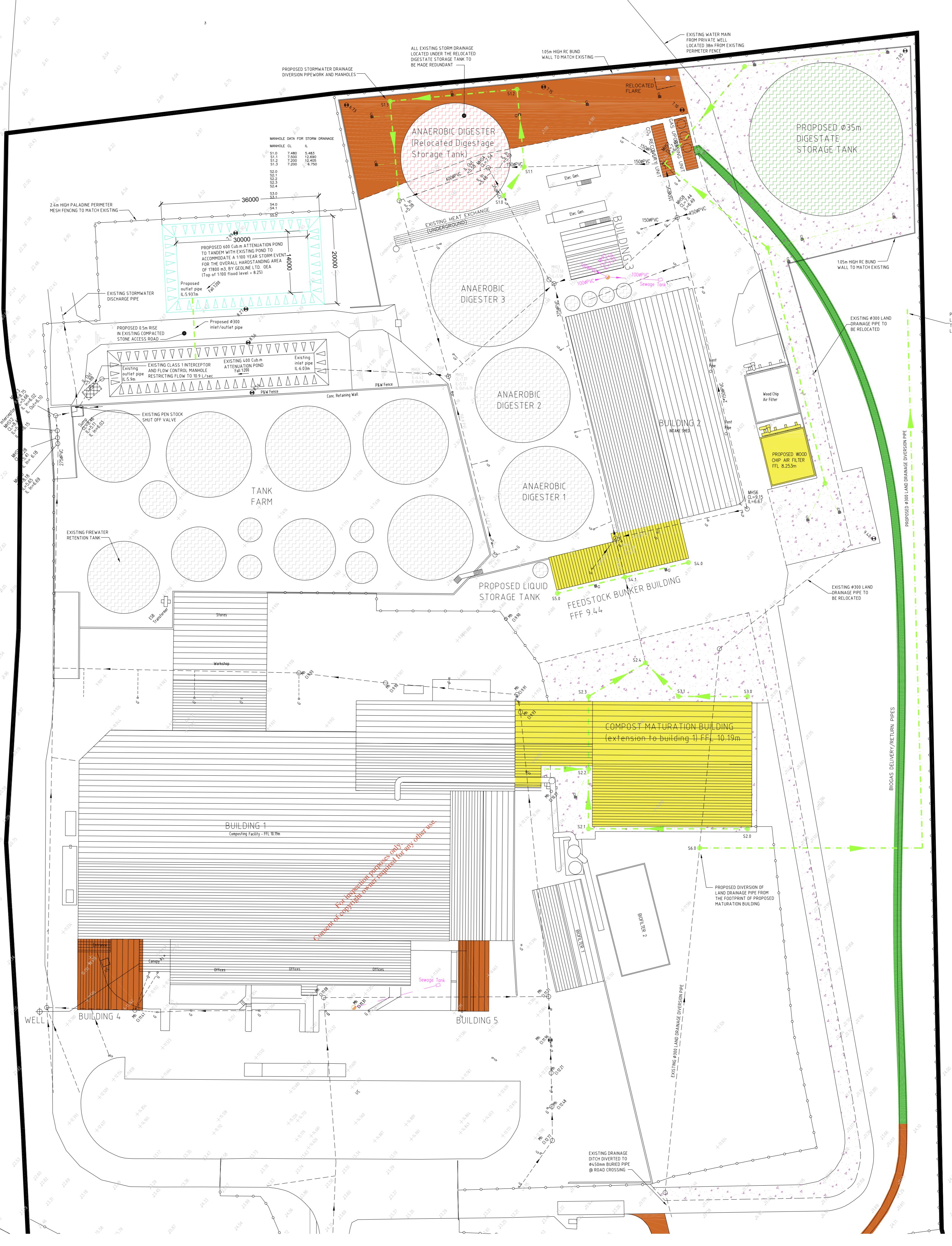
SITE DRAINAGE PLAN SCALE 1:500
