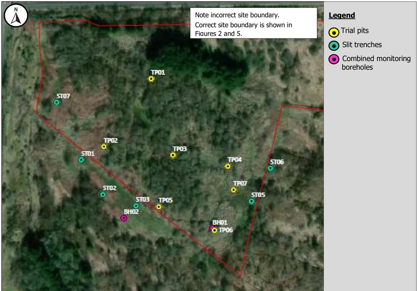
Figure 6: Trial pit (TP), slit trench (ST) and combined monitoring boreholes (BH)
