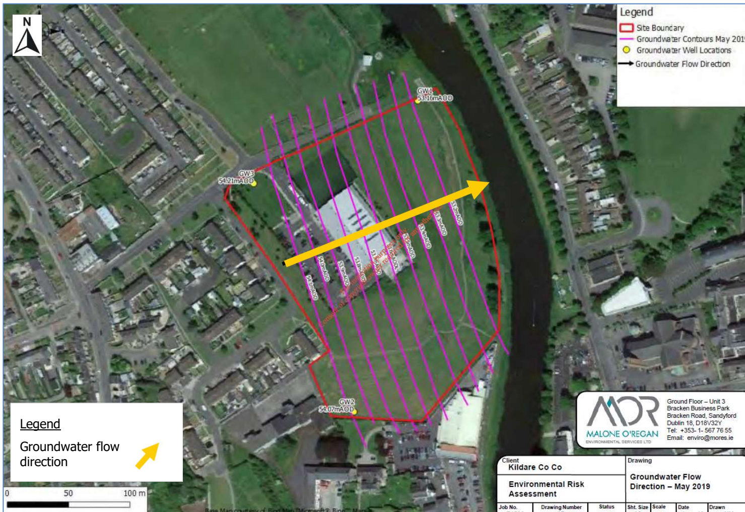
Figure 5: Groundwater flow direction
