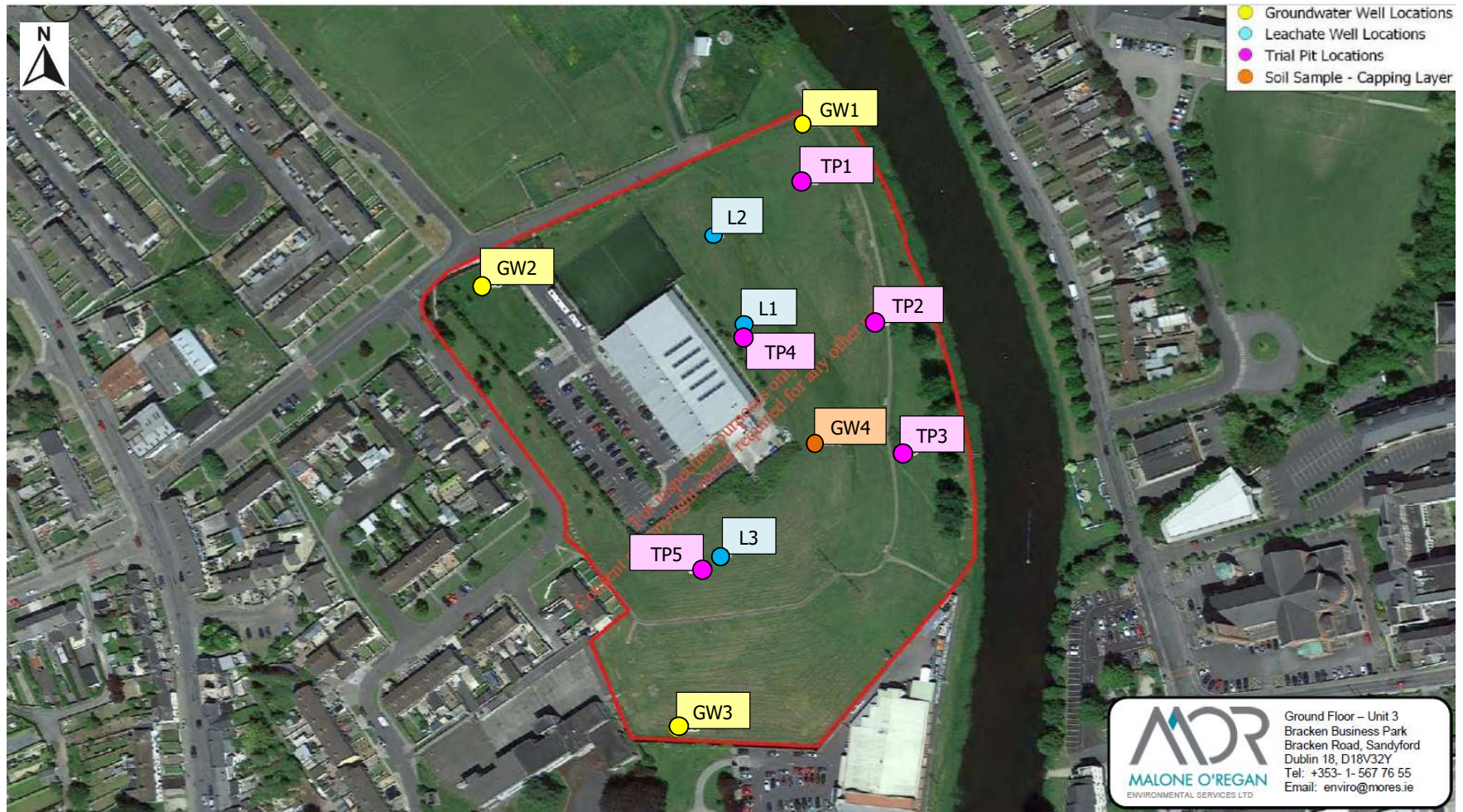
Figure 6: Groundwater well (GW), trial pit (TP) and leachate (L) monitoring locations
