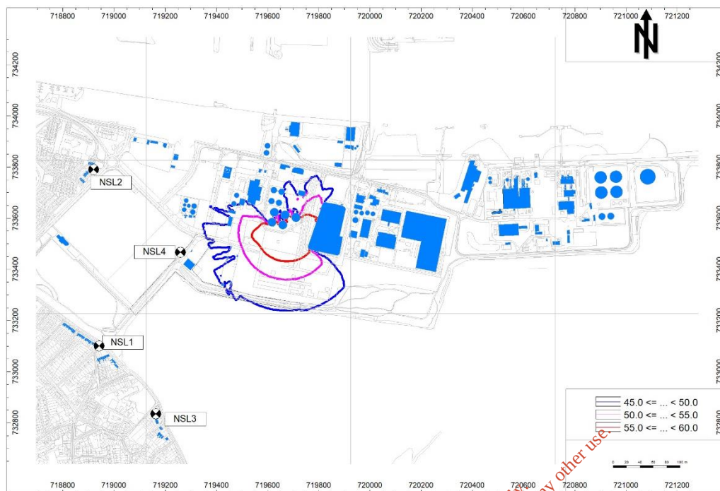
Figure 7.14: Operational Noise Contour Map – South Wall BESS
