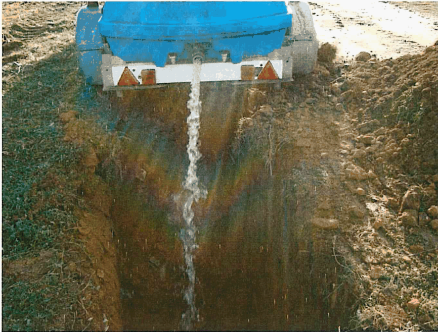
Figure 5. SA2 – Filling Testhole with water
