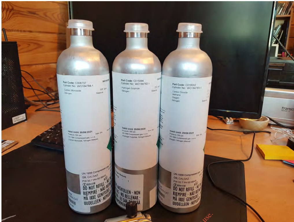
Plate A13.1 Gas mixtures and gas flow regulator used to pre/post calibrate the GA5000 Landfill Gas Monitor; Canister one- Carbon monoxide (CO), Canister two- Hydrogen sulphide (H 2 S) and Canister 3- Methane (CH 4 )
