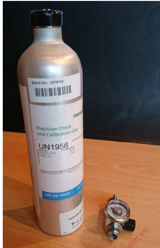
Plate A13.3 Gas mixture (Isobutylene) and gas flow regulator used to pre/post calibrate the MiniRAE3000;
