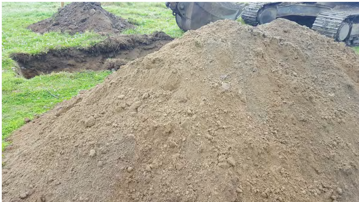
Plate 23. Stockpile of soil from trialpit, TP31 (i.e. note undisturbed indigenous SAND subsoil)
