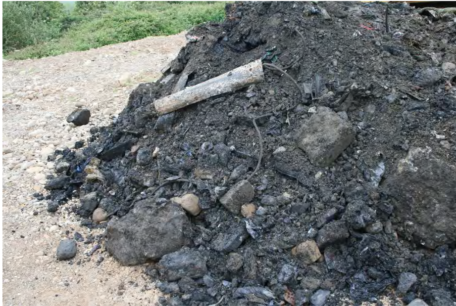
Plate 21. Typical stockpile of Type 2 waste (i.e. note grey/black coloration & high organic matter content, trialpit TP16 stockpile)
