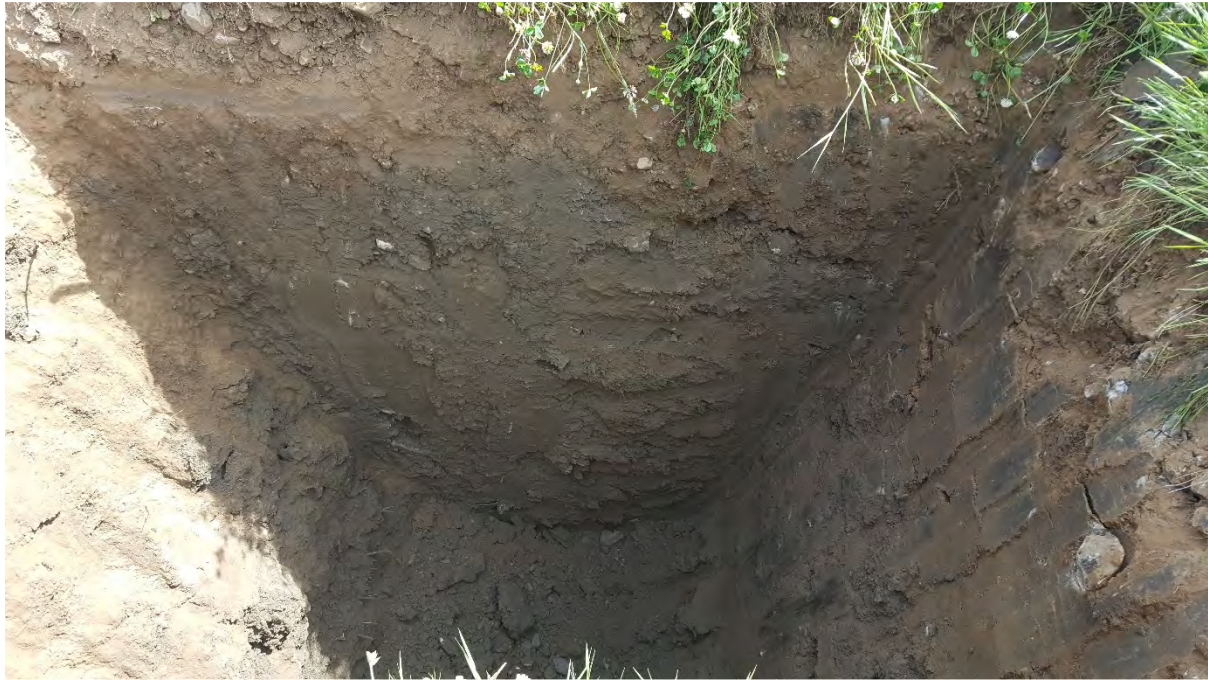
Plate 24. Soil profile of trialpit, TP25 excavated to the north of the builders compound (i.e. note absence of waste)
