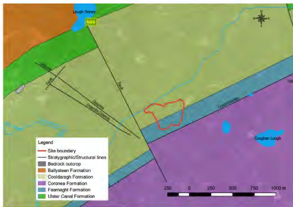
Figure 2.3. Bedrock geological map for the survey area (site indicated by red boundary).
