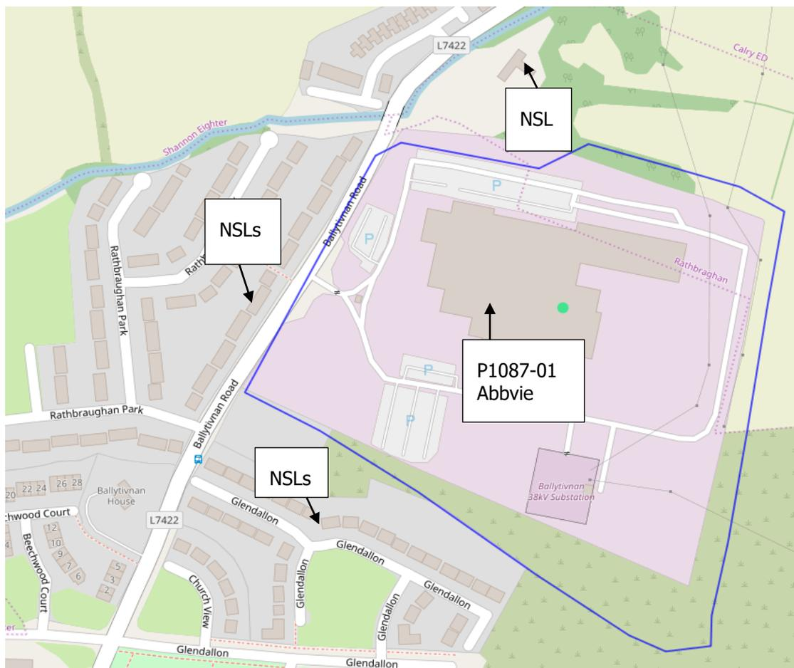
Figure1: Noise sensitive locations (NSLs) in relation to installation.
