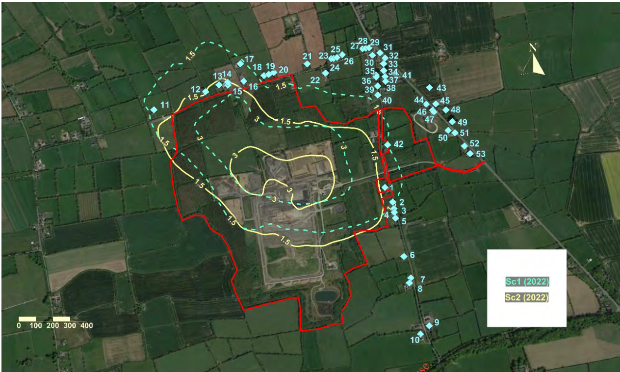
Figure 7-8: Predicted odour exposure levels for landfill operations for Scenario 1 (Year 4 do nothing) & Scenario 2 (Year 4 development)
