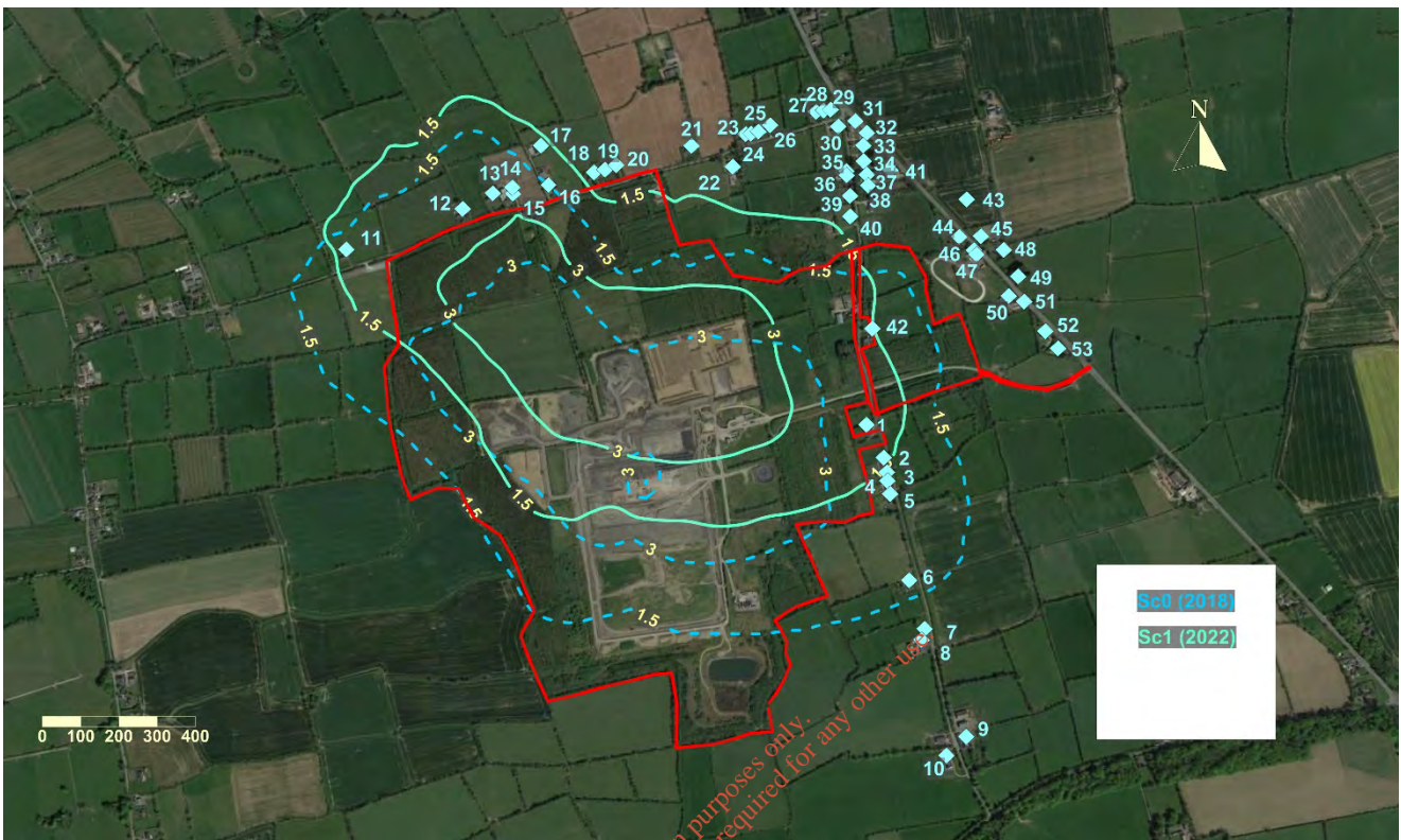
Figure 7-7: Predicted odour exposure levels from landfilling operations for Scenario 0 and Scenario 1 (Year 4 'do nothing')
