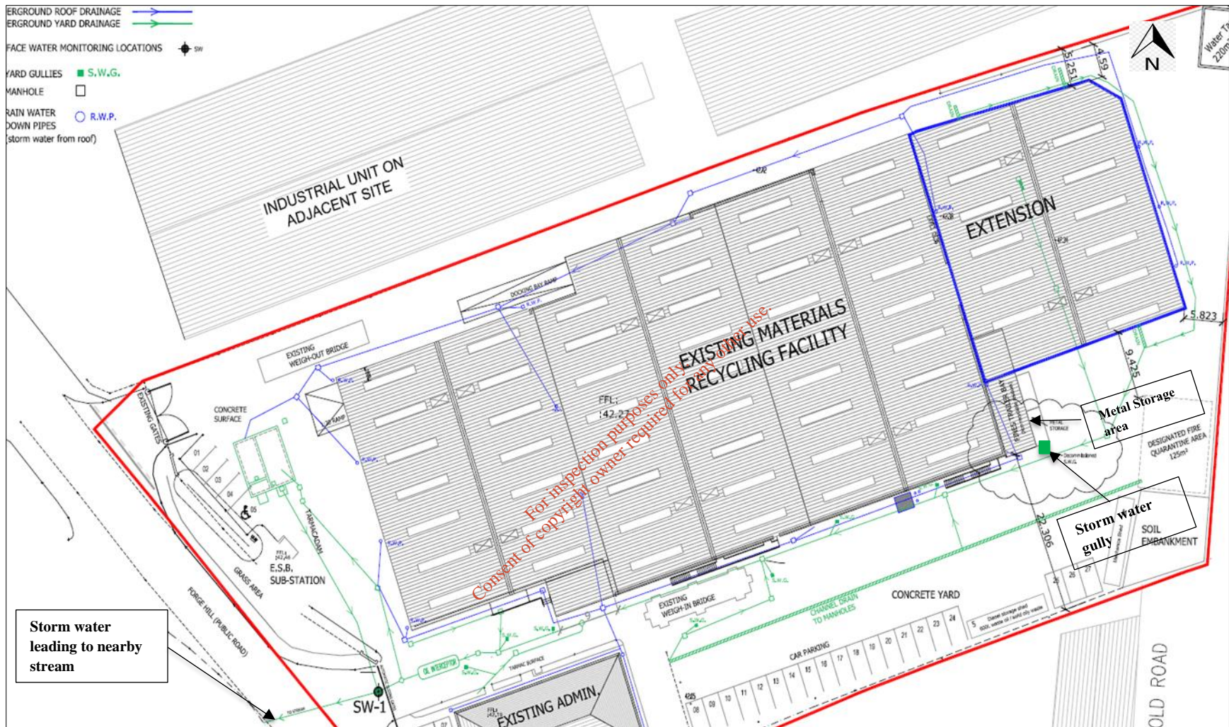
Figure 4. locations of Metal storage area, storm water gully and nearby stream (Source: Brian O’Kennedy & Associates Ltd)
