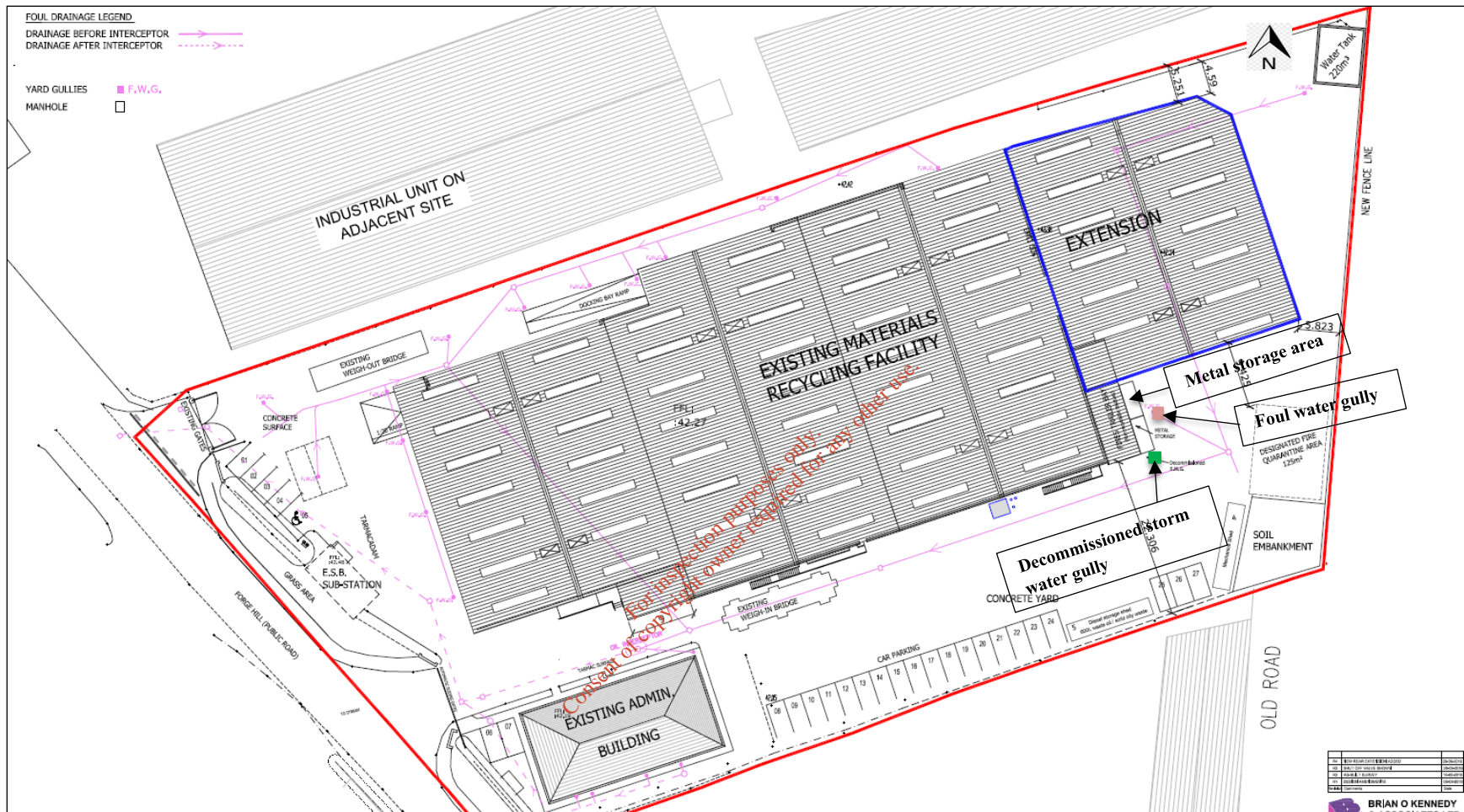
Figure 7. Location of metal storage area, foul water gully, metal storage area (Source: Brian O’Kennedy & Associates Ltd)
