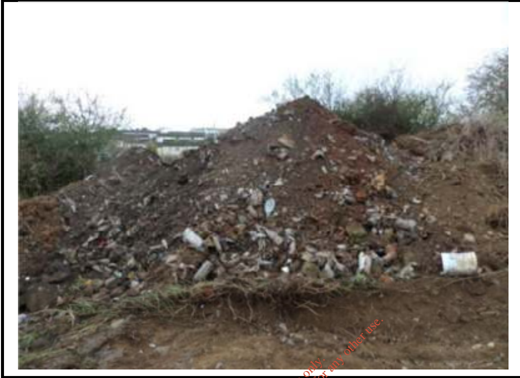
Photograph 13: Waste Contained in Trial Hole 12 (TH 12).
