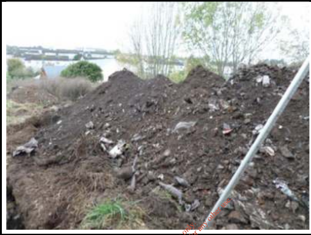
Photograph 10: Waste Contained in Trial Hole 9 (TH 9).
