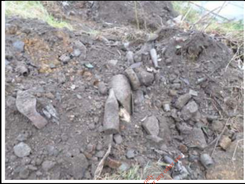
Photograph 4: Waste Contained in Trial Hole 3 (TH 3).
