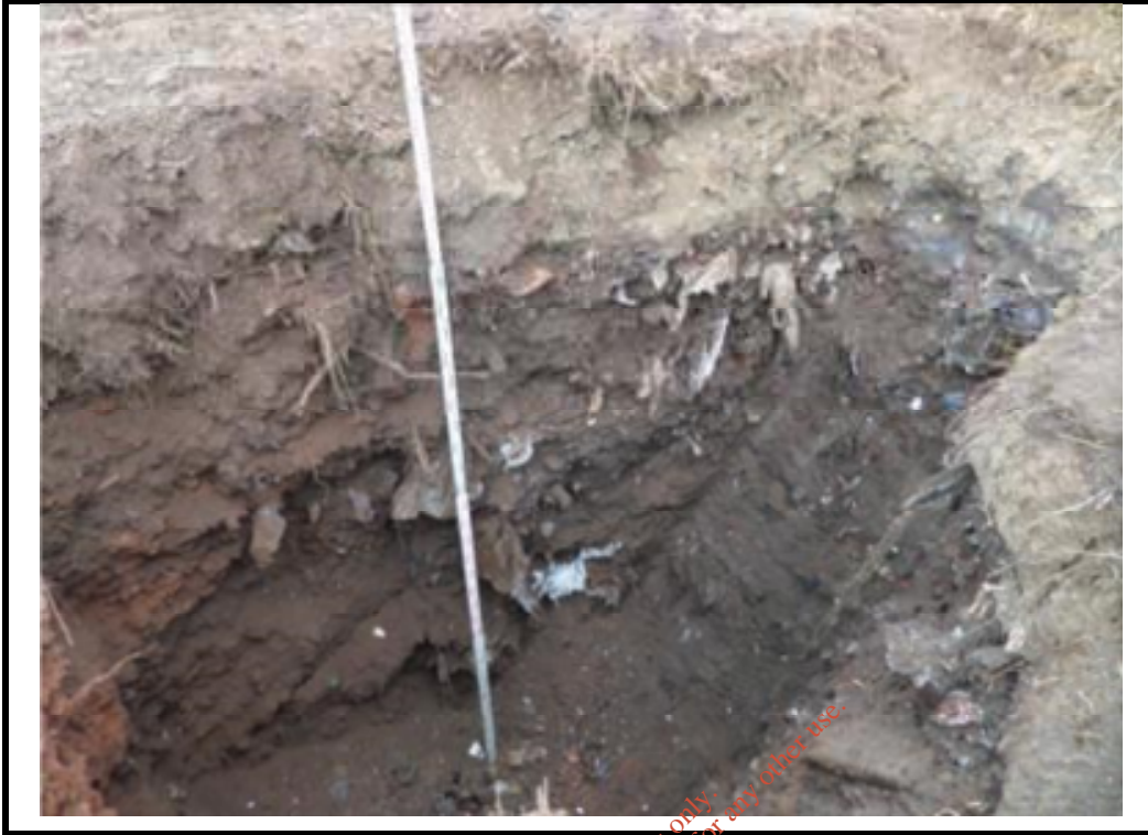
Photograph 18: Waste Contained in Trial Hole 23 (TH 23).
