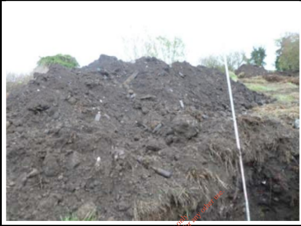
Photograph 6: Waste Contained in Trial Hole 5 (TH 5).
