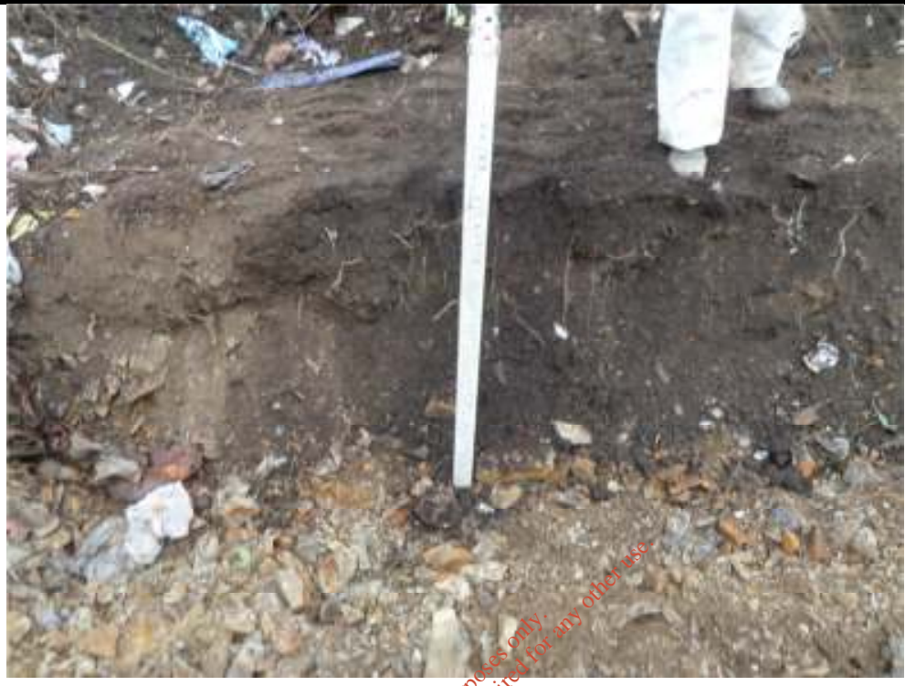
Photograph 22: Shallow Bedrock located in TH 17
