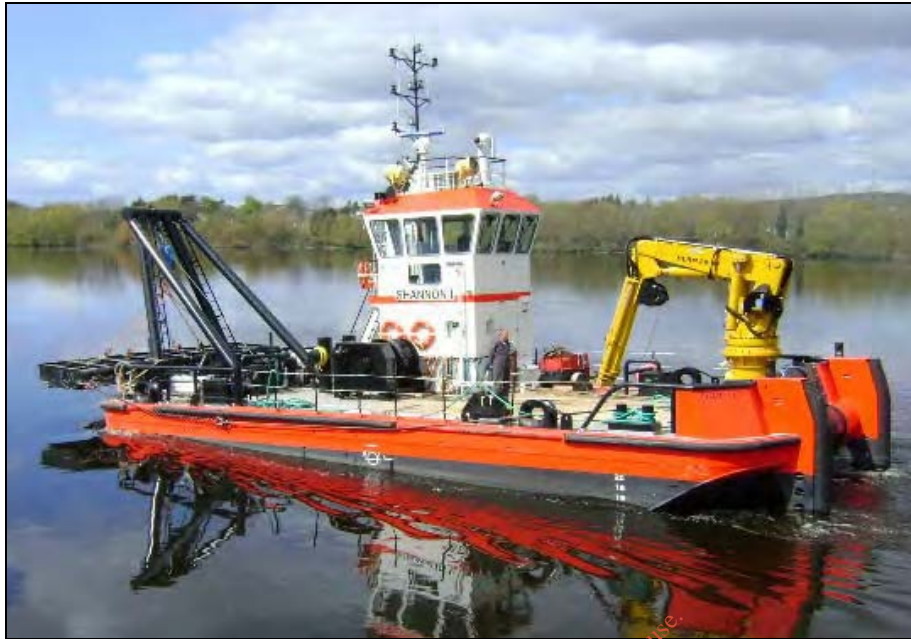
Photograph D.3-1 Multicat M.V. “Shannon 1” to be used for plough dredging at Limerick and also part of Foynes Port
