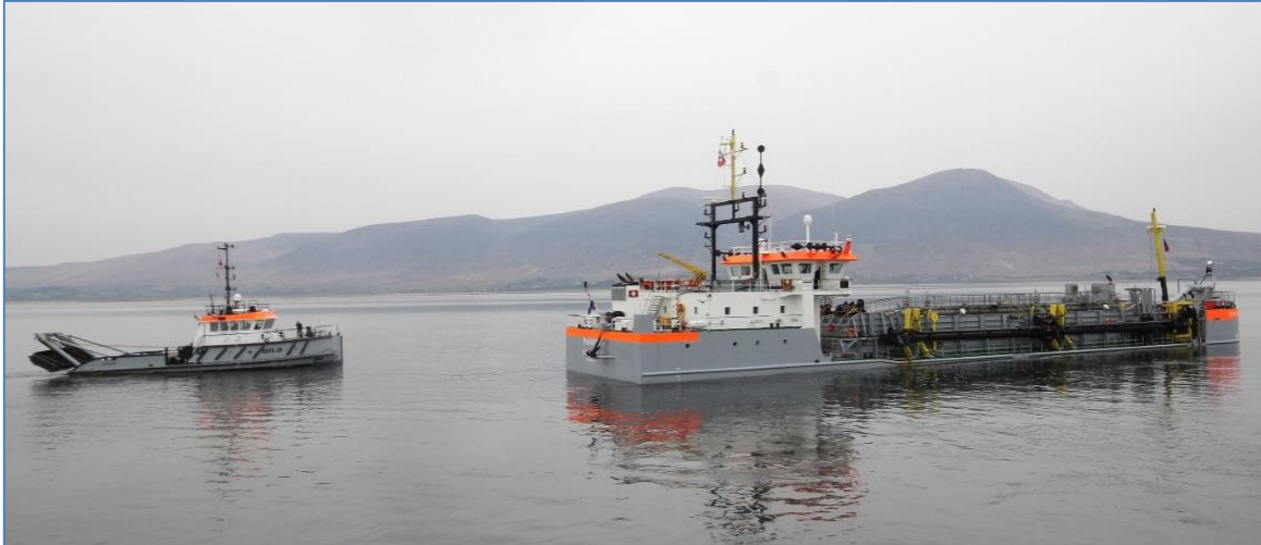
Plate 5: Survey and bed-levelling vessel Kees Jr. on left and suction dredger vessel Mahury operating at Fenit.
