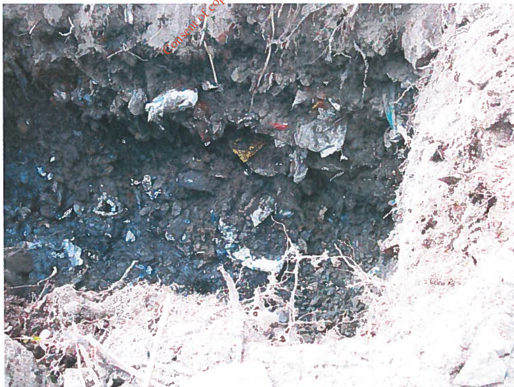
Photo 2: waste very dry and decomposed
