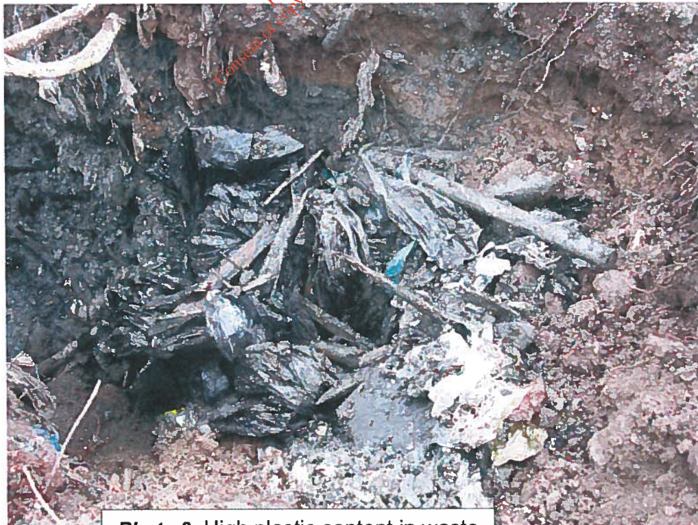
Photo 2: High plastic content in waste
