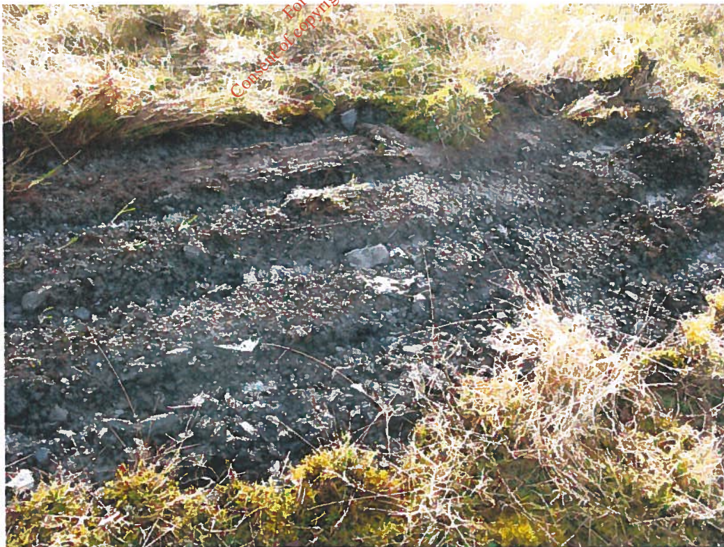
Photo 7: Trial Hole 2 with leachate at base
