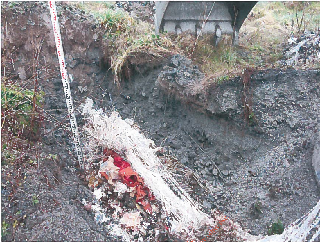
Photo 1: Commercial Waste at 1 metre
