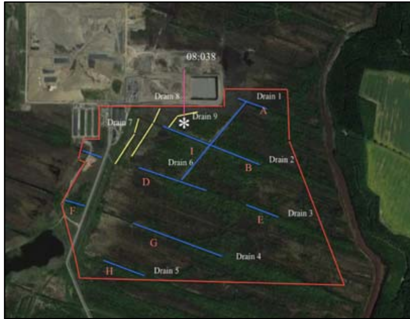
Fig. 4: Aerial view of site indicating the location of drains cleaned (Blue) and more recently excavated drains (yellow) with the location of KD008:038 also highlighted.
