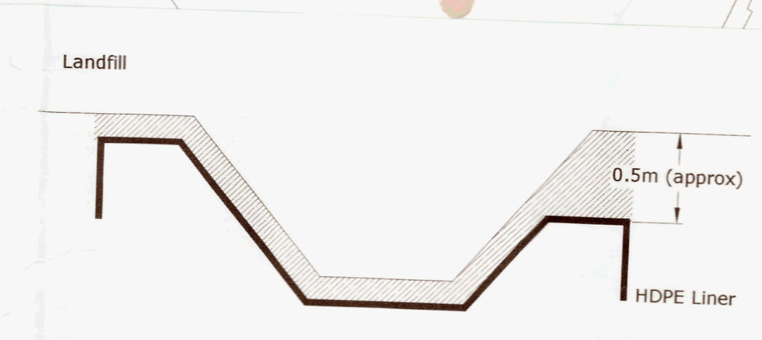
DETAIL B DETAIL OF WORKS TO DRAINAGE DITCH, NORTHERN BOUNDARY OF SITE (NOT TO SCALE)
